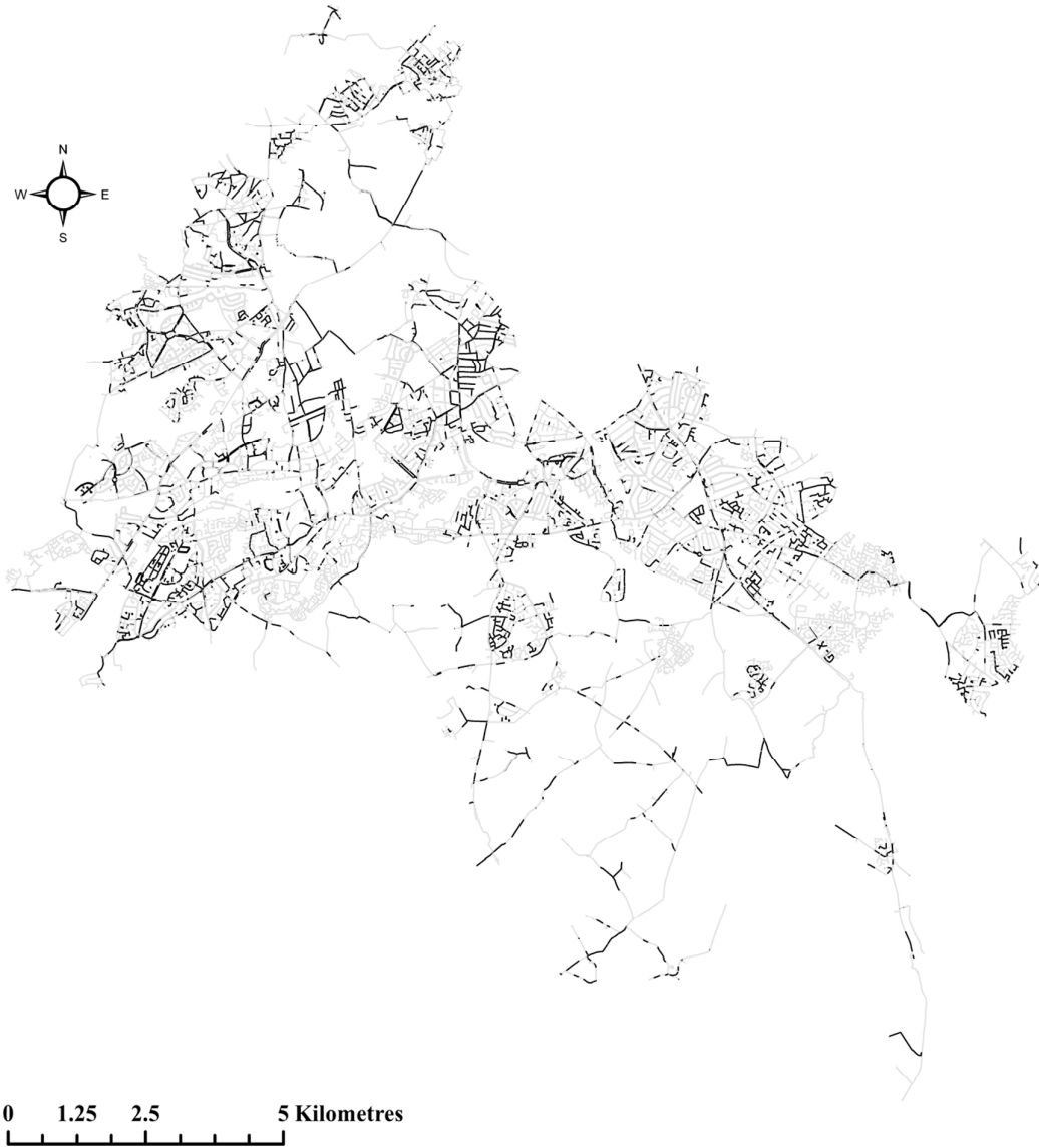
Figure A.3 EPR predictions of pipe failure rate in wrong ranges (black pipes)
