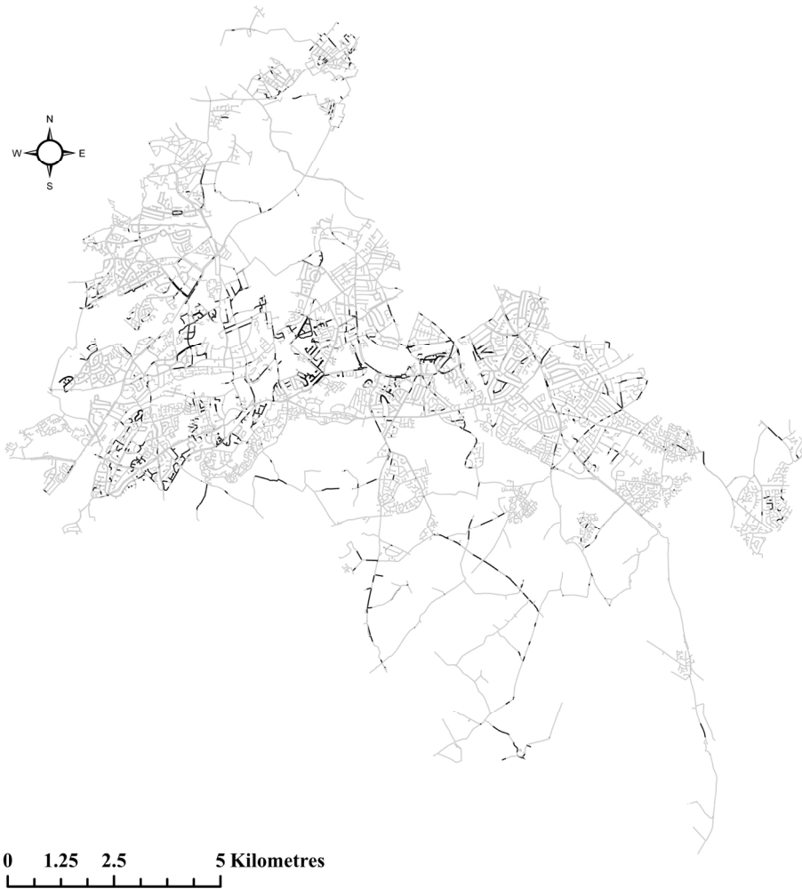
Figure 6. Six-clustered EPR predictions of pipe failure rate in wrong ranges (black pipes)
