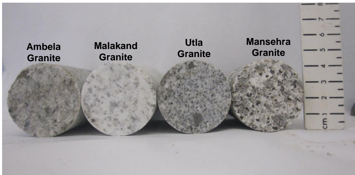
Figure 3.3. Characteristic granite samples from NW Pakistan used in current investigation for mechanical testing.
