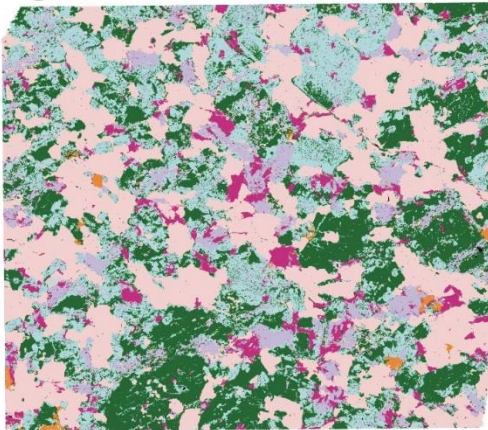
Fig. 7.3. Representative mineral maps of studied granites generated via QEMSCAN analysis.
