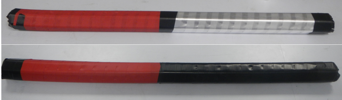
Figure 5.13: P1-16* and P1-17* anti friction membranes as installed prior to testing. Top image: P1-16* (Left: 1 x layer of Dacron. Right: 2 x layers of Endumax tape TA23). Bottom image: P1-17* (Left: 2 x layers of Dacron. Right: 2 x layers of Bell Plastics Black UHMWPE).
