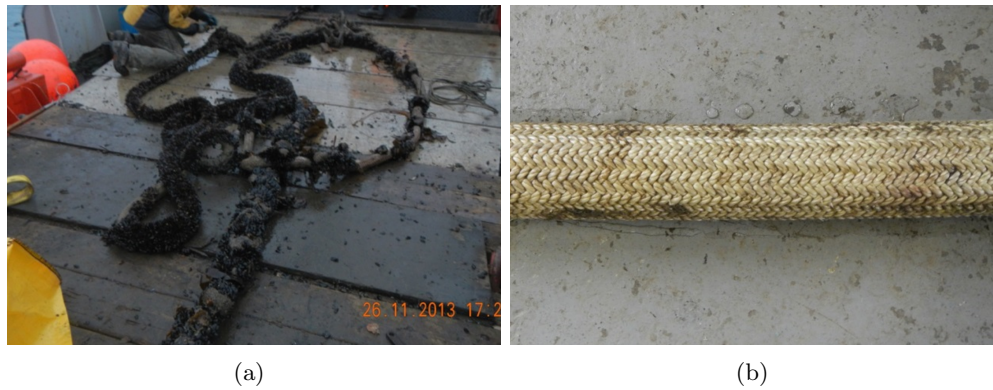
Figure 5.29: (a) Upper tethers with significant marine growth following sea deployment; (b) tether P1-8 following cleaning with a bristle brush and fresh water
