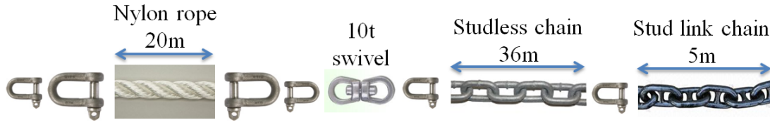
Figure 3.1: Graphical representation of a typical mooring limb design from SWMTF. A combination of 9.5t and 25t D shackles are used to link different components of the mooring system. From left to right the mooring is aligned from top to sea bed.
