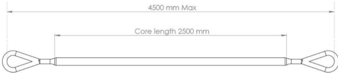
Figure 2.34: Exeter Tether dimensions detailing core length. Note total length has some variation but maximum length of 4500mm (image not to scale). Replicated from Gordelier et al. (2015).
