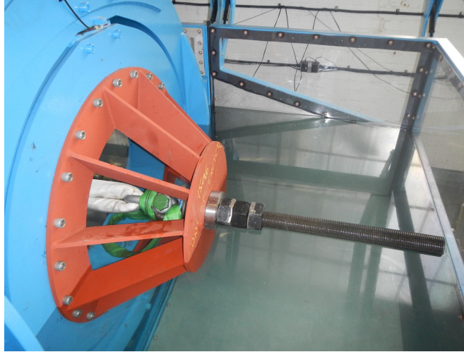
Figure 3.9: DMaC pre-tension adjuster which enables slack to be removed from the system and a pre-tension to be set prior to dynamic testing.
