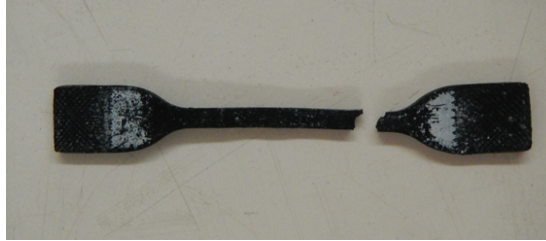
Figure 5.37: Example of a rejected sample for the ISO37 test procedure; the failure occurred too close to the end of the sample.
