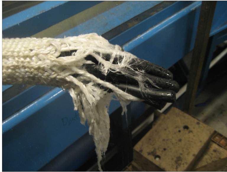
Figure 5.16: TLL failure of tether P1-16. Failure occurred during the 1% - 70% NWBS load range and on the 176 th cycle.
