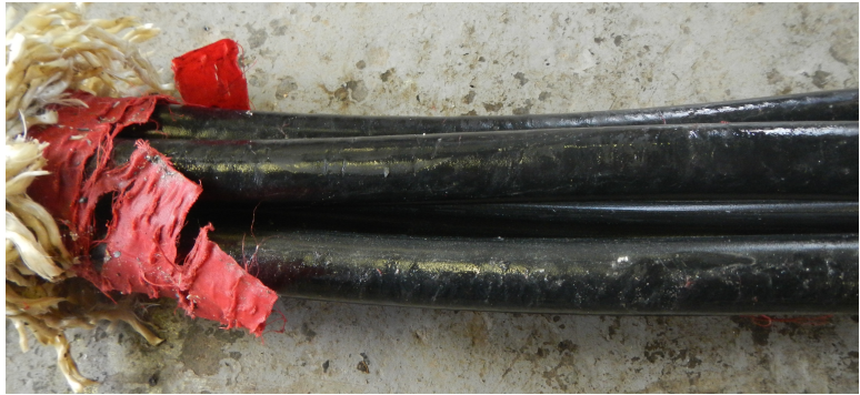
Figure 5.34: Elastomer core following sea deployment showing minor compression deformations on the outer surface of the strands.
