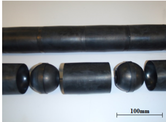
Figure 2.33: Articulated Core construction detailing moulded female and male double hemisphere components assembled (top) and exploded (bottom).
