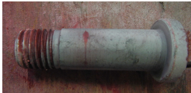
Figure 4.25: Shackle fatigue crack identification using DPI. Fatigue crack as developed on Shackle 7 at 27,976 cycles.
