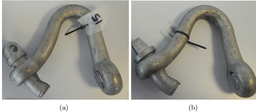
Figure 4.23: Ultimate strength failure modes. (a) Shackle A and (b) Shackle B.
