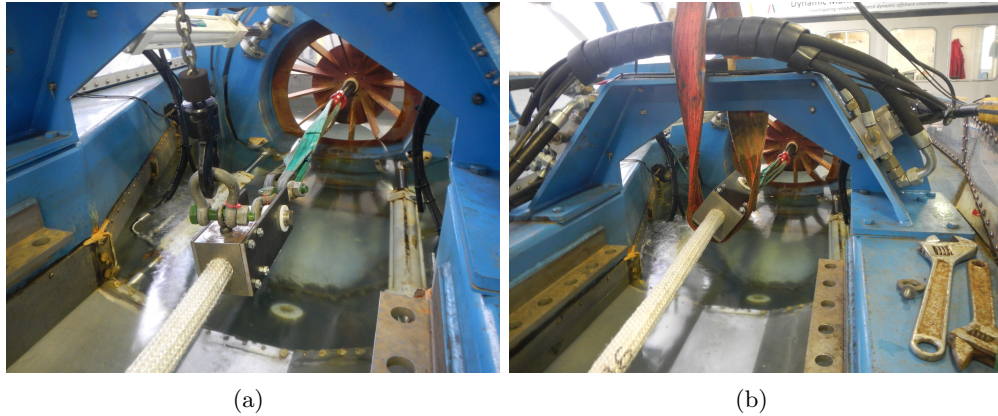
Figure 5.15: Rope collet arrangement in situ during anti friction membrane durability testing. (a) details original arrangement using a hook through the eye bolt but this was found to introduce too much twist into the tether set up; (b) details the final arrangement with a strop to support the collet, this arrangement was used for the testing.
