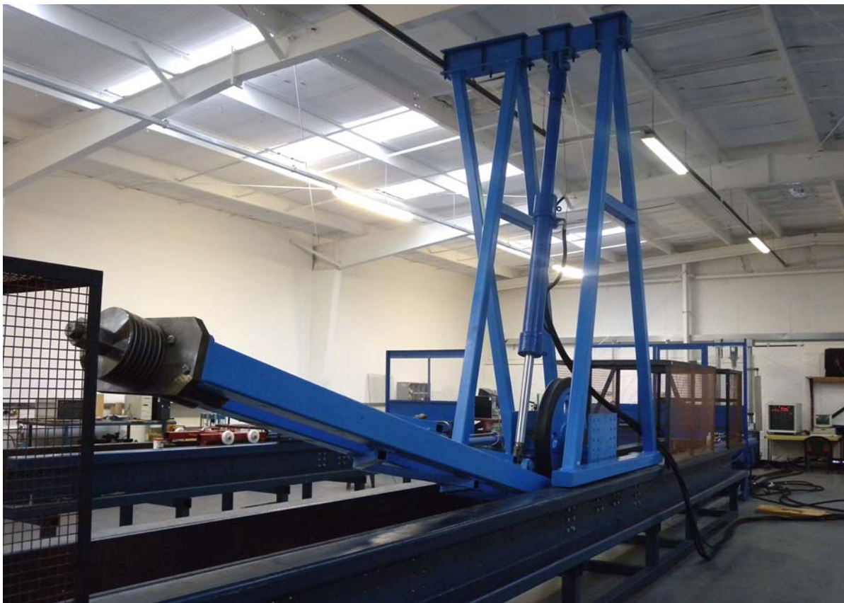
Figure 10 Cyclic Tension and Bend Test Machine, TTI Labs, Wallingford
