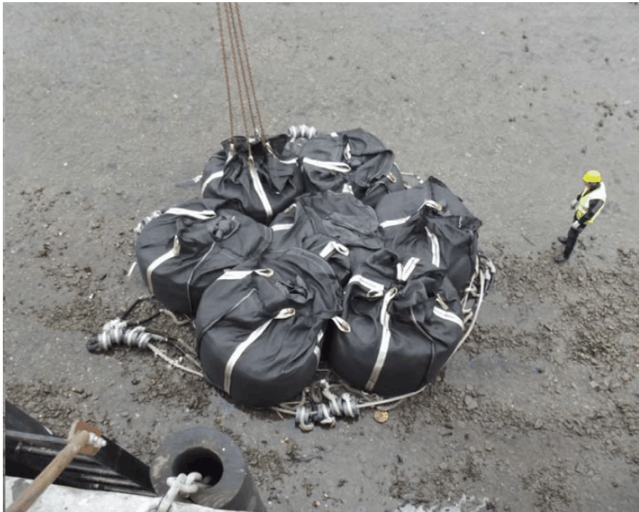
Figure 12 Prototype Bag Anchor System on Harbor Seafloor, Isle of Man, for Pull Tests
