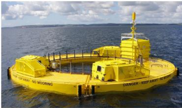
Fig. 2. Field examples of systems to test loads related to MRE devices. (a) South West Mooring Test Facility (SWMTF), (b) SWMTF mooring configuration [12], and (c) Fred Olsen BOLT Lifesaver device.
