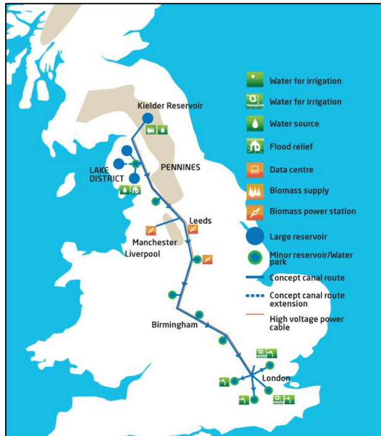
Figure 8.2: Map of proposed national water grid between North and South UK (map taken from the Chartered Institute of Building, (2013))
