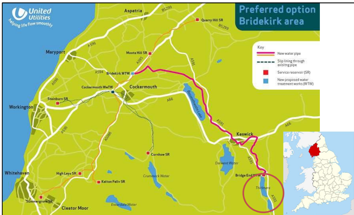
Figure 8.1: Map of proposed interconnecting pipeline option for West Cumbria (image adapted from United Utilities (2014))
