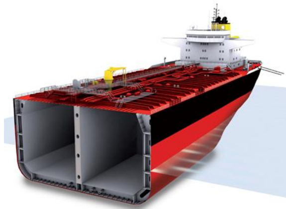
Fig 2.6 Cross section of double hull tanker
