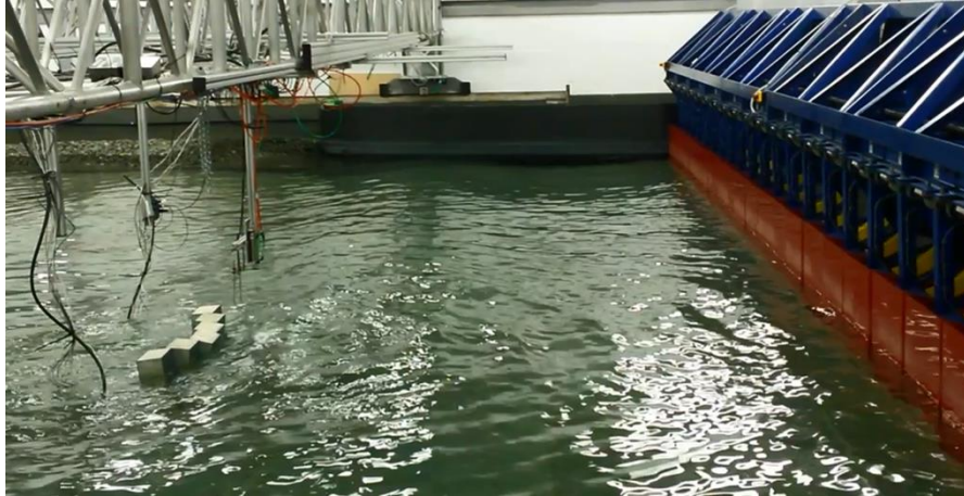
Figure 3. Photograph of the physical model, in its Modular Flap configuration, operating in the wave tank.
