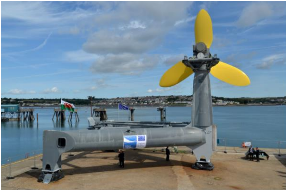
Figure 4-1: Constructed 400kW full scale prototype Tidal Energy Ltd DeltaStream device.
