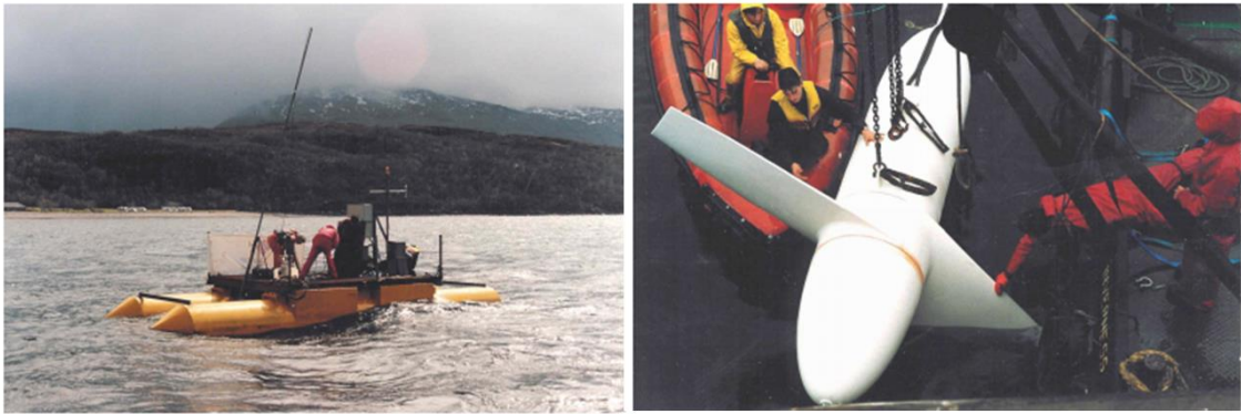
Figure 2-6: The first tidal turbine, a 15kW proof of concept device, as developed by IT Power Consulting Ltd, deployed and tested in 1994 in Loch Linnhe, Scotland. Images copyright of Marine Current Turbines Ltd, sourced: http://www.british-hydro.org/ .
