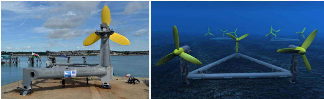
Figure 3-3: TEL Ltd DeltaStream device, left) constructed 400kW full scale prototype, right) artist impression of 1.2MW DeltaStream. Images copyright of TEL Ltd, sourced: www.tidalenergyltd.com .
