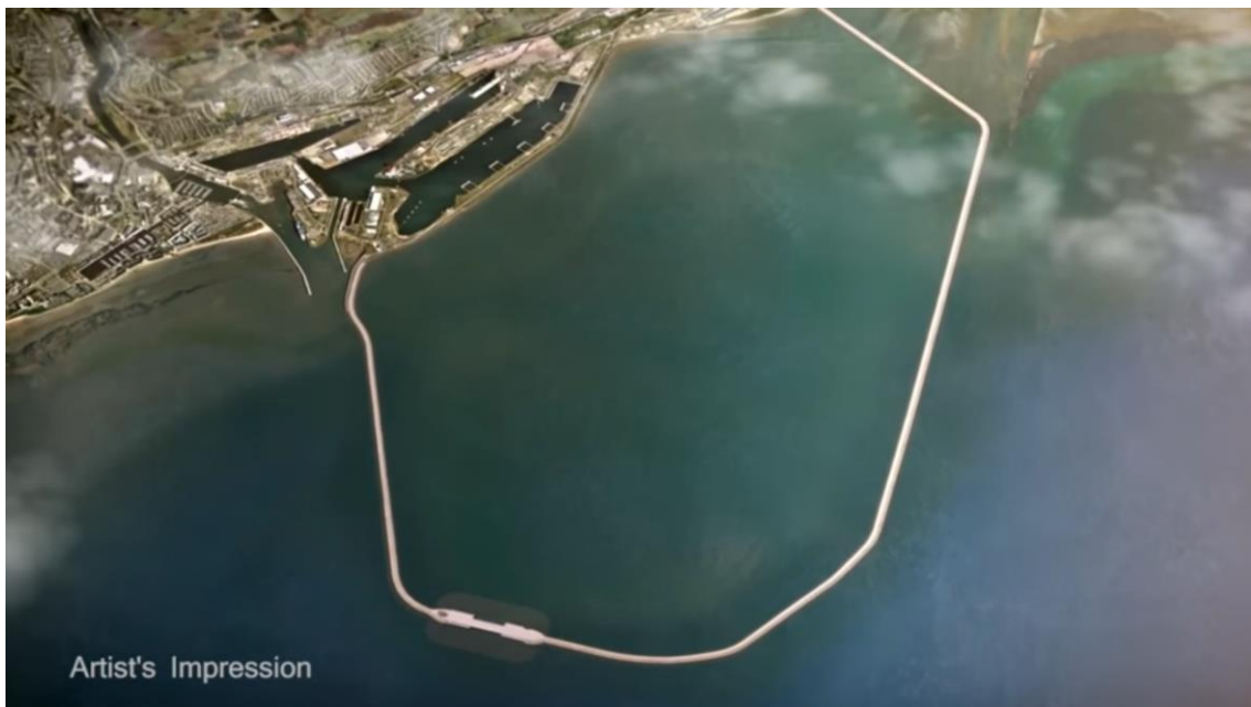
Figure 2-5: Artist's impression of the 320 MW Swansea Bay tidal lagoon. Image copyright of Tidal Lagoon Power, access from www.tidallagoonpower.com .
