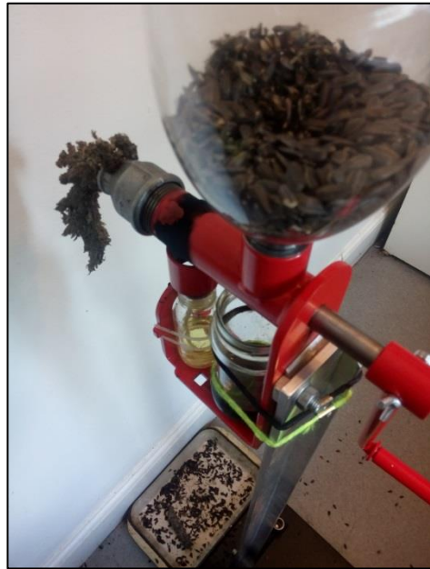
Figure 23: The oil press in action
