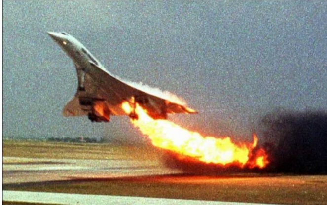
Fig.4-5. Air France Concorde Flight 4590 seconds after take-off. A piece of debris on the runway was flicked up by one of the aircraft's wheels at nearly 300kmh. It pierced a wing fuel tank, causing a fire, loss of the aircraft and 113 lives. (Source: Buzz Pictures/Corbis Sygma)
