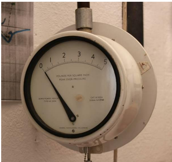
Fig.7-33. A Bomb Power Indicator – on loan from the ROC Museum (now defunct) to Great Bedwyn post. As the respondents noted (above) this item is now worth £1000. (Source: Bob Clarke 26/05/2012)
