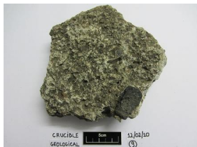
Figure 6.49 - Geological sub-types G2 (top) and G3 (centre and bottom). Note the crucible fragments adhering to the G3 example (bottom).
