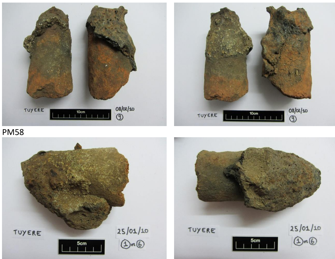
Figure 6.30 - Tuyere fragments sub-type T1. Note the angled vitrification and the large vitrified clay lump with finger marks (bottom).
