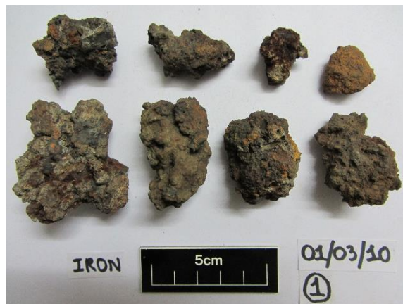
Figure 6.52 - Iron sub-types I1 (top), I2 (centre) and I3 (bottom). Note the dendritic or coral iron nature of the I1 lump (top).
