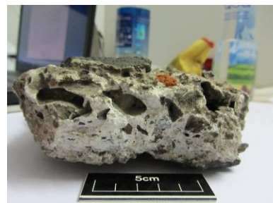
Figure 6.49 - Geological sub-types G2 (top) and G3 (centre and bottom). Note the crucible fragments adhering to the G3 example (bottom).
