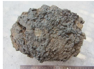
Figure 6.6 - Tap slag sub-type TS2. Note the top surface protrusions on the large TS2 fragment (bottom).
