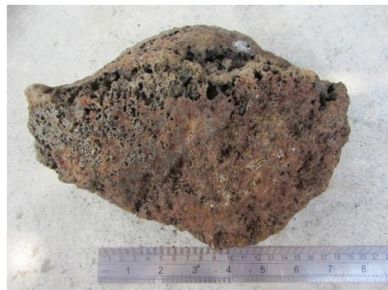
Figure 6.18 - Furnace slag sub-type FS6. Note their very porous honeycomb-like nature and the remnants of the original surfaces in the form of a thin crust (bottom).
