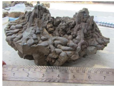
Figure 6.6 - Tap slag sub-type TS2. Note the top surface protrusions on the large TS2 fragment (bottom).
