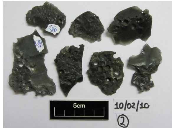
Figure 6.44 - Glassy slag sub-types GS1 (top) and GS2 (bottom). Note the colour variation from grey to glassy green on the GS1 fragments (top) and the bulbous top side and flat porous underside of the GS2 fragments (bottom).
