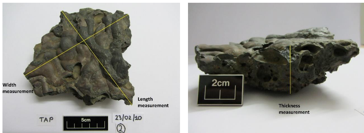
Figure 4.2 - Measurements taken for the slag fragments. Similar measurements taken for the ore, metal and geological fragments.
