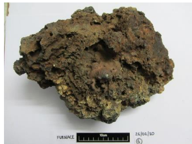
Figure 6.14 - Furnace slag sub-type FS2 (top) and FS2.1 (centre and bottom). Note the rough broken surfaces of the FS2 slag (top), the well-rounded projections on the FS2.1 slags and the adhering tuyere fragment (bottom).
