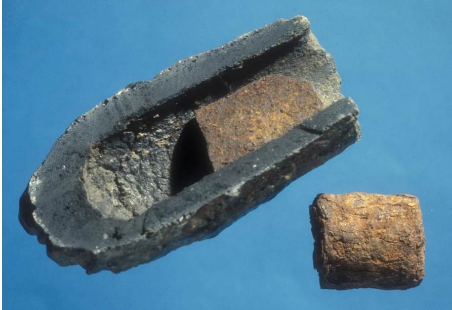
Figure 2.3 – Crucible section and bloom fragments recovered from Mawalgaha (photo courtesy of G. Juleff).
