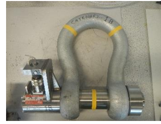
Fig 3: A 55t load shackle with bespoke pin fitted with strain relief bracket and signal amplifier.
