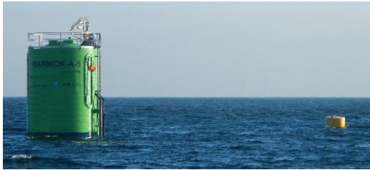
Fig 1: The MARMOK-A5 device deployed at BiMEP. One of the pennant buoys supporting a corner node is visible on the right hand side of the photo.
