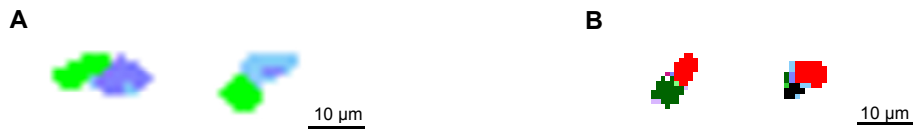
Figure 4.20: Difference between the liberation and association of the valuable minerals within the <10\ \mu\text{m} size fraction. (A) apatite (green) and (B) synchysite/parisite (red).
