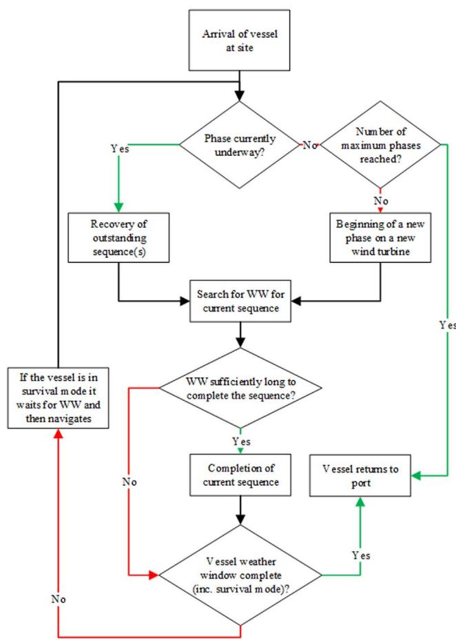
Fig. 3.3. Flowchart of logistical process.
