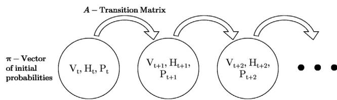
**Fig. 3.1.** Schematic representation of the Markov Chain: Wind Speed ( $V_t$ ), Wave Height ( $H_t$ ), Current Speed ( $P_t$ ).
