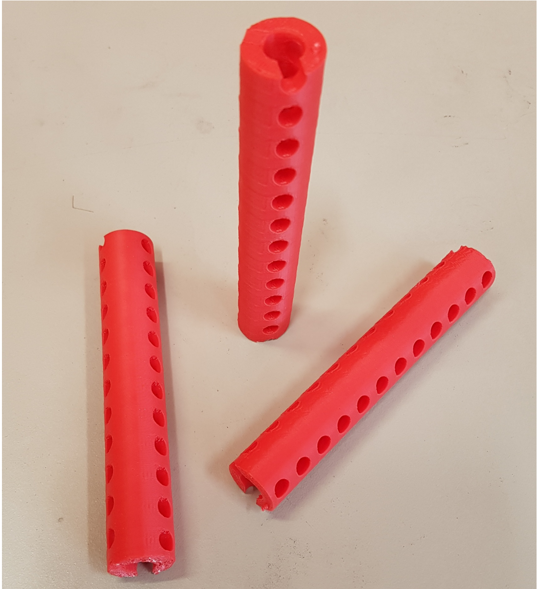
Figure 9.6: Picture of unassembled sample with screw-symmetry, printed by the 3D-prototype machine.
