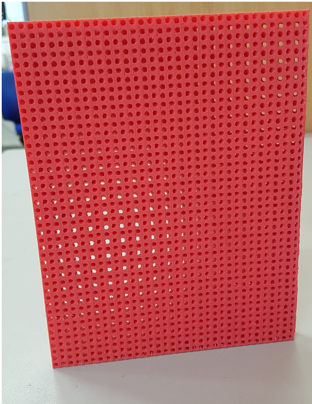
Figure 9.8: Picture of 3D-prototype printed sample, consisting of a square lattice of open-ended cylinders. Each unit cell contains 4 cylinders, and each cylinder is ‘twisted’ so that they emerge in a different location on the surface plane of the exit side than on the entrance side.
