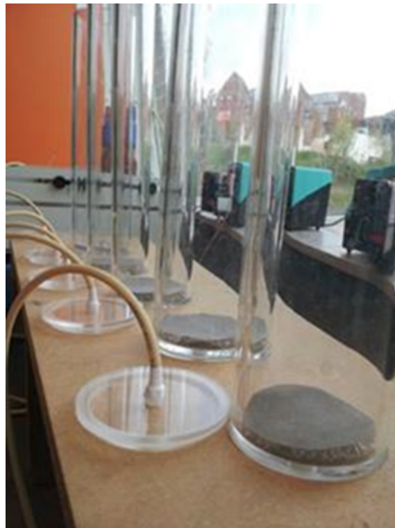
FIGURE 4.3: Photographic image showing the set up of the quartz sand columns prior to packing. One layer of glass beads and a layer #60 mesh stainless steel installed at the bottom and repeated again (in reverse) at the top of each column to ensure an even distribution of flow.
