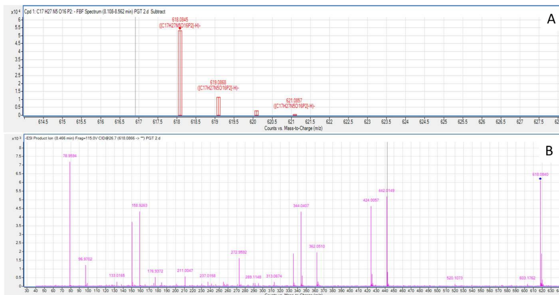
Figure 38: Accuracy score for GDP-6dBep from Q-TOF scan in negative mode. (A) Find By Formula spectrum of for C 17 H 27 N 5 O 16 P 2 . Red boxes show isotopes; red lines denote observed isotopes. (B) expected fragments from GDP-6dBep.
