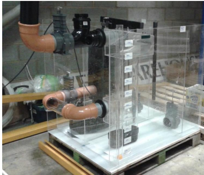
Figure 5.4.2 – Test rig used to measure the discharge rates for a range of outlet orifices
