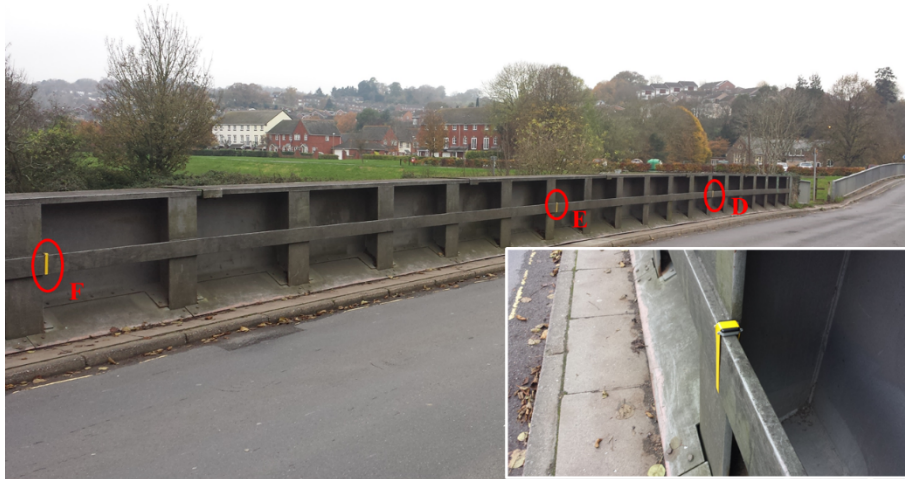
473 Fig. 9, IMUs deployed at sensor locations F, E & D (see Fig. 7), insert shows how IMUs were simply 474 taped to the horizontal member adjacent to the vertical web stiffener.
