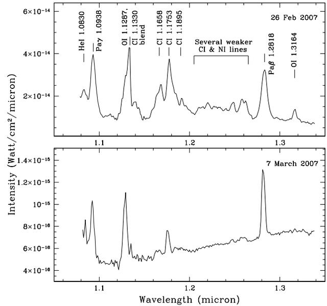
**Fig. 4.** J band spectrum of V1280 Sco on February 26.97 ( $t=22\text{d}$ , top panel) and March 7.95, 2007 ( $t=38\text{d}$ , bottom panel) are shown. The prominent emission lines are marked. The formation of dust between the two epochs is evidenced clearly from the rising of continuum towards longer wavelengths in the later spectrum of 7 March 07, while no dust signature is visible in the first spectrum.
