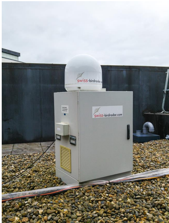
Figure 1. The Birdscan MR1 system on the roof of the Environment and sustainability Institute building at the University of Exeter. The device is compact and can be sited in any location provided its line of sight is not blocked by other structures or vegetation. Photograph: Greg Wills, University of Exeter.
