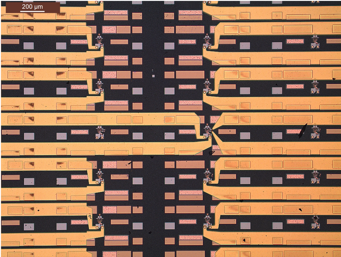
(a) Micrograph of a wafer section showing the gold traces to which one copy of each writer is connected
