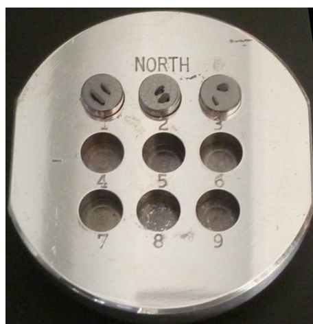
Figure B-7. SEM sample holder with 3 stubs holding shell fragments.
