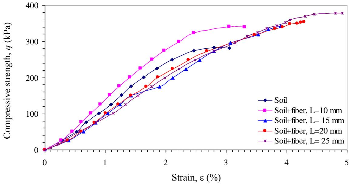
**Fig. 2.** Stress-strain curves for natural soil and reinforced soil with 0.5% fiber and different lengths
