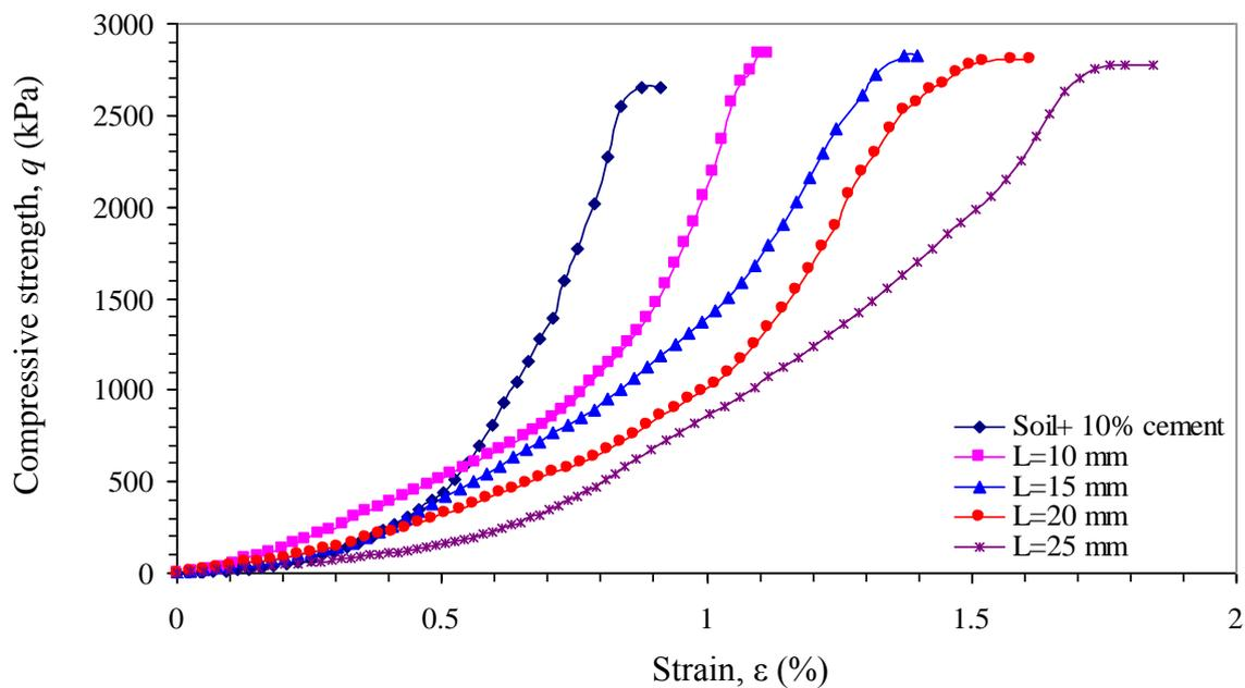
**Fig. 5.** Stress-strain curves for soil-cement and reinforced soil-cement with 10 % cement and 0.5% fiber for curing time of 28 days
