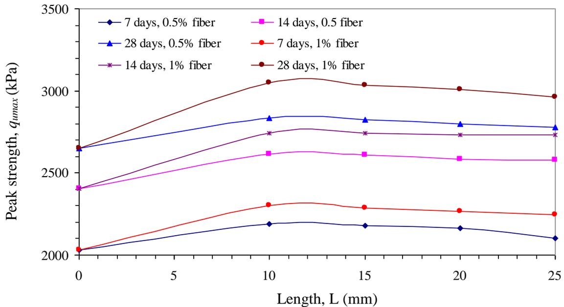
**Fig. 7.** Variations of peak strength against length of fiber for soil-cement with 10 % cement and fiber inclusion of 0.5% and 1% at different curing times
