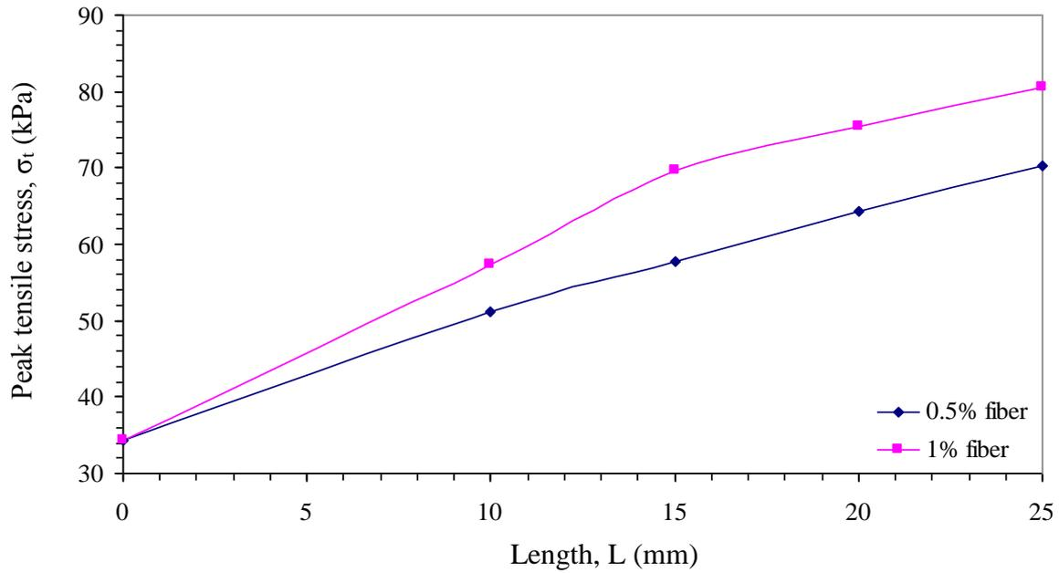
**Fig. 10.** Variations of peak tensile stress against length of fiber for reinforced soil samples with 0.5 and 1% fiber content
