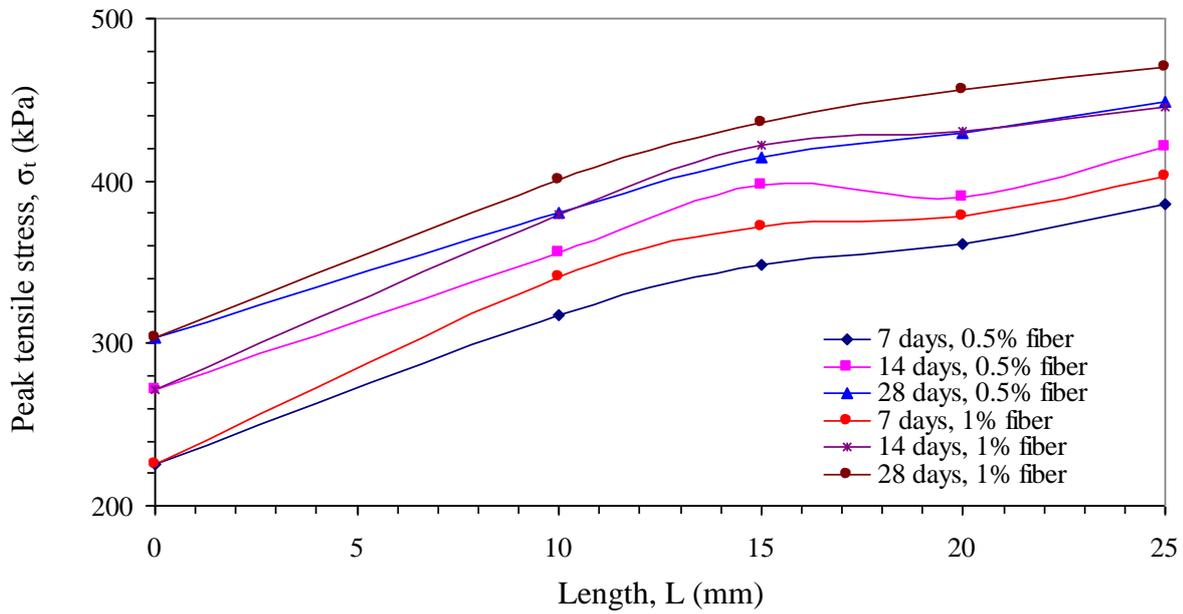
**Fig. 12.** Variations of peak tensile stress against length of fiber for reinforced soil-cement samples with 10% and 0.5 and 1.0 % fiber inclusion at different curing times
