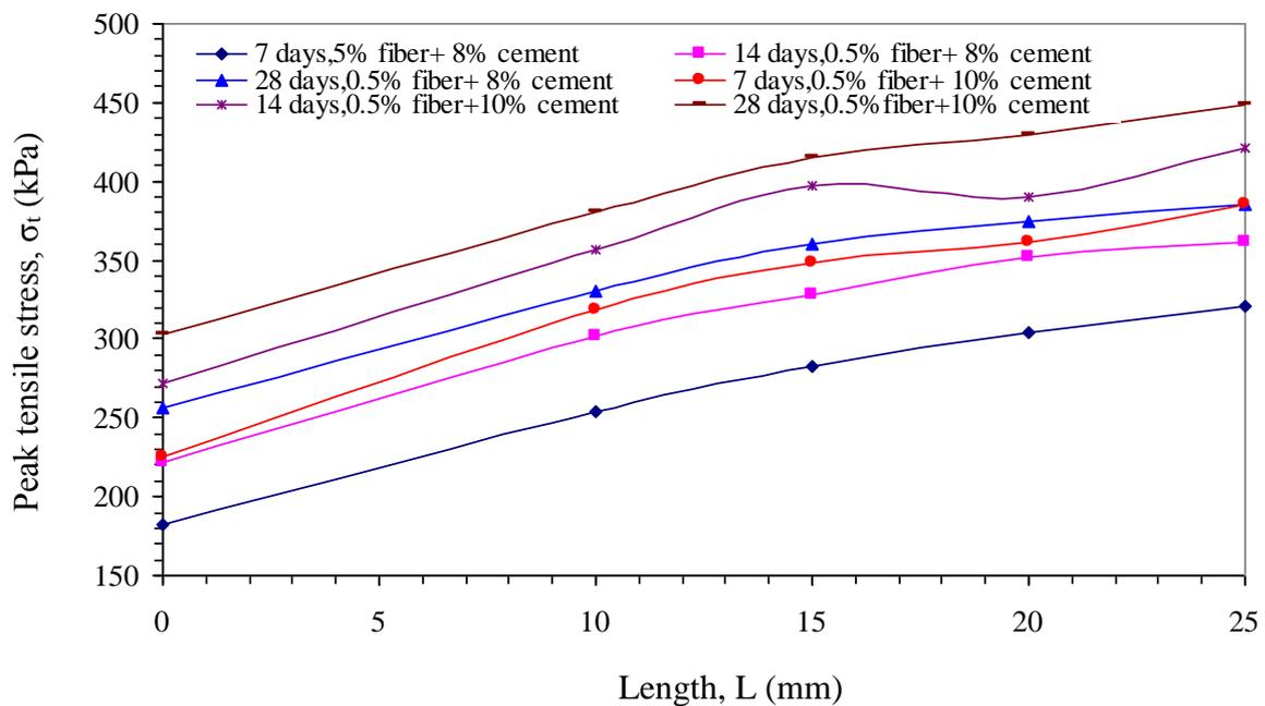
**Fig. 11.** Variations of peak tensile stress against length of fiber for reinforced soil-cement samples with 8 and 10% cement at 0.5 % fiber content
