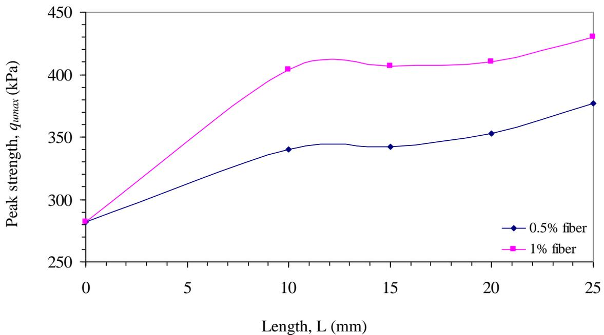
**Fig. 3.** Variations of peak strength with length of fiber for 0.5 % and 1% fiber content
