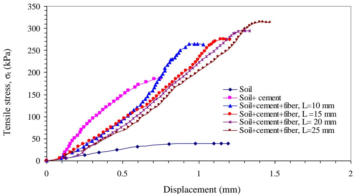
**Fig. 9.** Tensile stress-displacement for soil, soil+8% cement and reinforced soil+cement with 0.5 % fiber at different lengths
