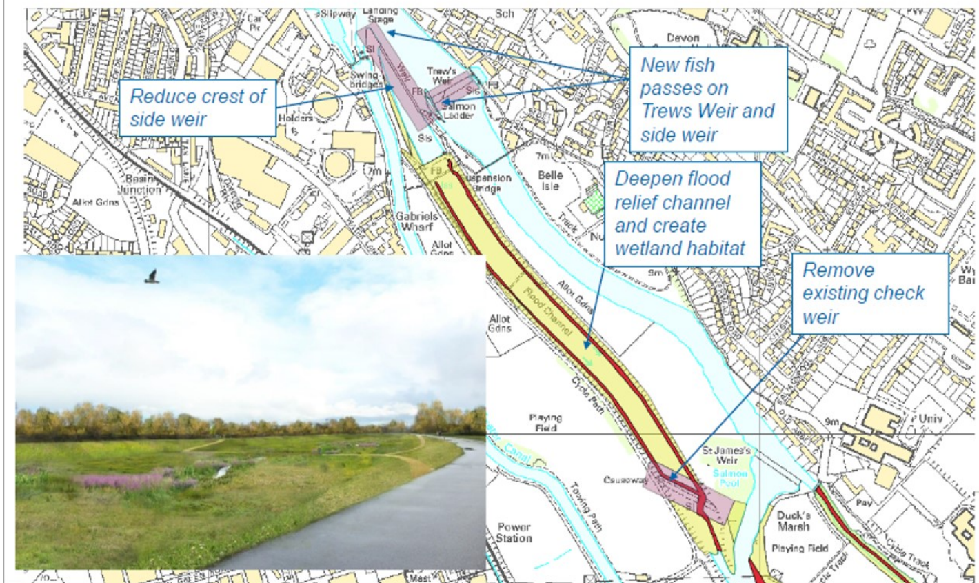
Figure A.4: Phase 1 of the upgrades on southern section of the Exeter flood defence scheme completed in 2016.
