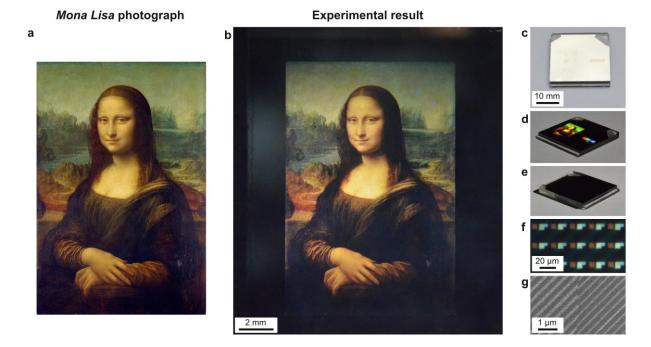
Figure 2. Experimental results showing images of an R<sub>VH</sub> device under various illumination conditions.
