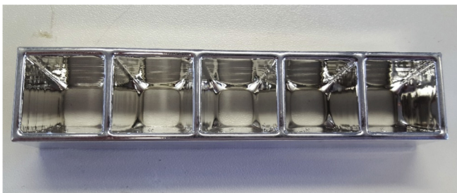
Fig. 6. Optics manufactured using 3d printing and evaporative coating.
