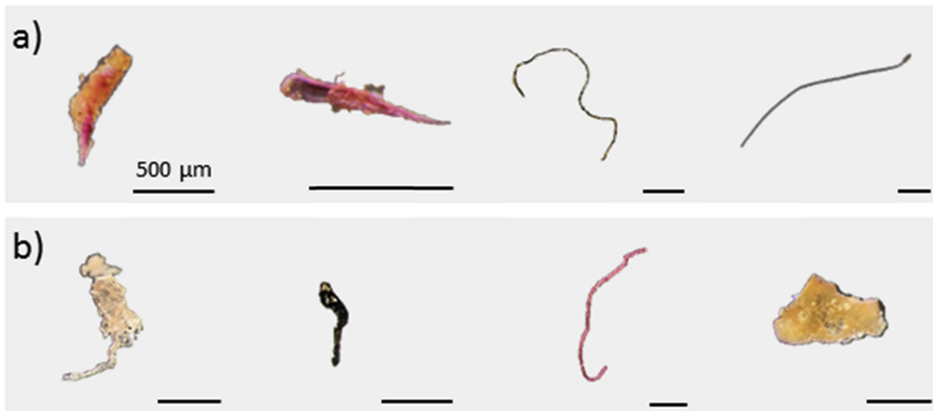
Fig. 2. Photographic examples of particles found in a) fish (from 1–r: aramid woven fabric, polyethylene, ethylene propylene, polyacrylamide) and b) scat subsamples (from 1–r: polyethylene, polyaramid Kevlar®, polypropylene, polyacrylamide). Scale bars represent 500 \mu\text{m} .
