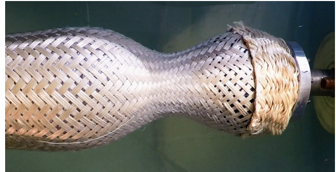
Figure 12. Waisting and bellying of the braid fibre with original 32 strand braid observed at 300 kPa during testing
