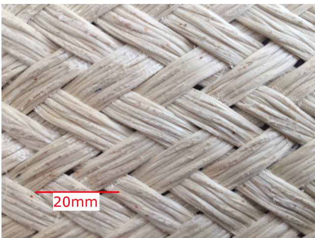
Figure 11. Detail of braid fibres after 500 000 cycles
