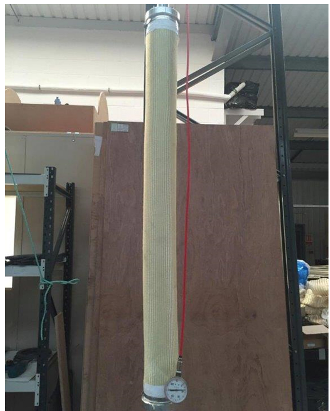
Figure 13. Fine weave braid after endurance testing
