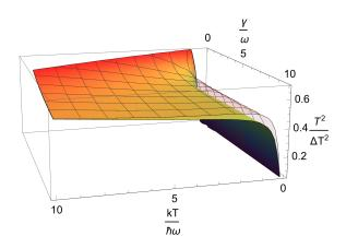
FIG. 2. Bound on temperature signal-to-noise ratio. Plot of the optimal signal-to-noise ratio of an unbiased temperature estimate,  $(T/\Delta T_s)^2_{opt}$  (coloured), as a function of T and  $\gamma$ . The mesh plot shows the upper bound given by (16).
