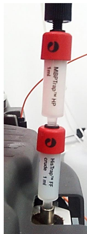
Fig.5.1: The arrangement of the MBPTrap and HisTrap columns used for the PinLip purification protocol 2.
