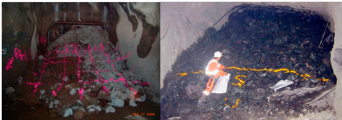
Figure 7. Drawpoint with sampling grid (Left) and sample collection (Right).
