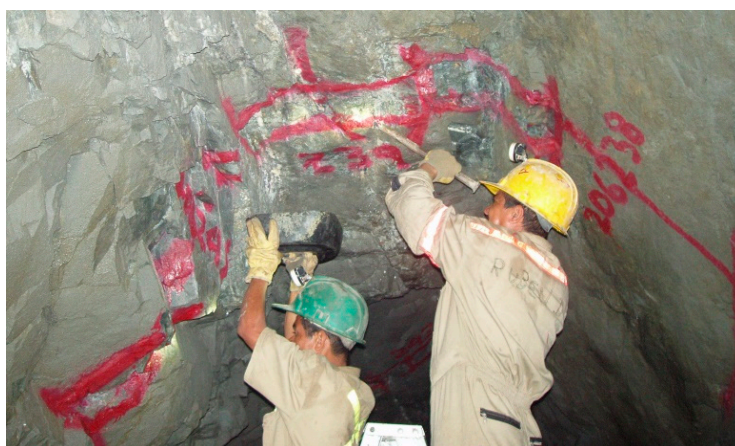
Figure 9. Backs channel sampling in historical workings. A chip-channel is produced, where sample fragments are supposedly being collected in a plastic bowl. In this case the EE is high, as many extracted fragments are not being collected. In addition, DE on the shoulders of the drive is particularly high since the delimited samples are biased within the delimited zone on the curved drive shoulder.
