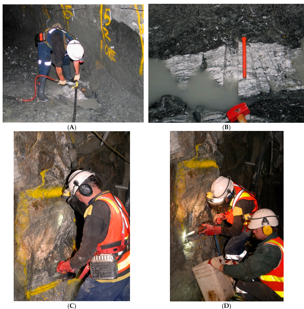
Figure 4. Collection of saw-cut channel sample (A) and resulting channel (B); Cutting a sidewall channel sample (C) and using an air pick to remove the sample (D).
