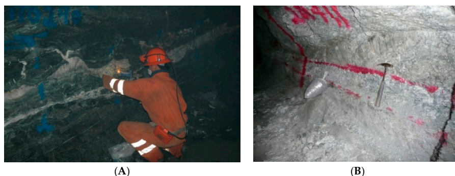
Figure 2. (A) Chip-channel sampling. Samples collected from sidewall of shanty drive. Each sample comprises near continuous chips collected across the vein; (B) Hand channel sampling of side walls.
