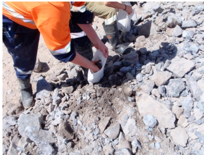
Figure 6. Grab sampling from a surface stockpile showing the challenges of collecting a representative sample and oversampling fine material.
