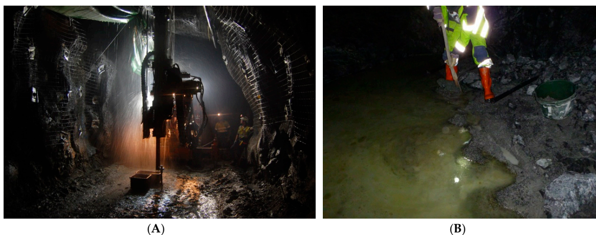
Figure 8. Types of sludge sampling. (A) Collection of stope blasthole sludge via plastic boxes placed below the hole leads to very high DE and EE; (B) Collection of face blasthole sludge via scooping from the drive floor leads to high FSE, GSE, DE, and EE.
