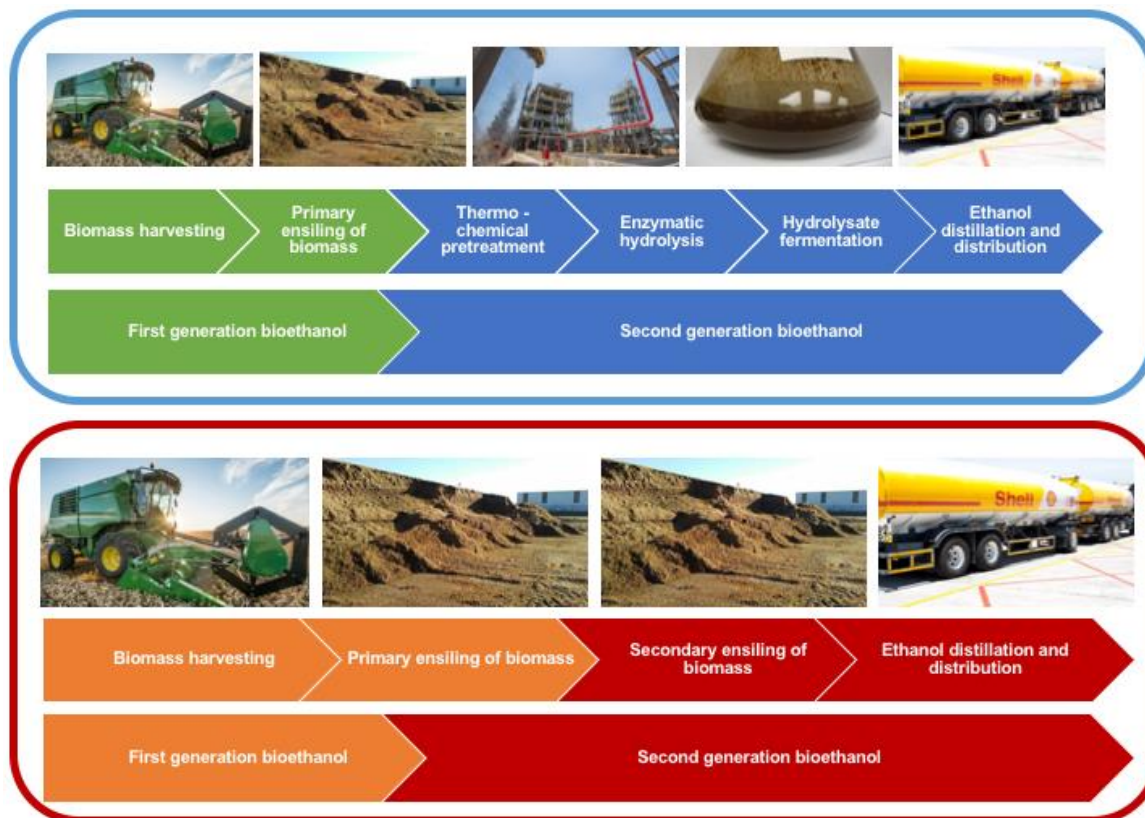
Figure 2. Comparative workflow of the two processes involved in the production of second generation ethanol
