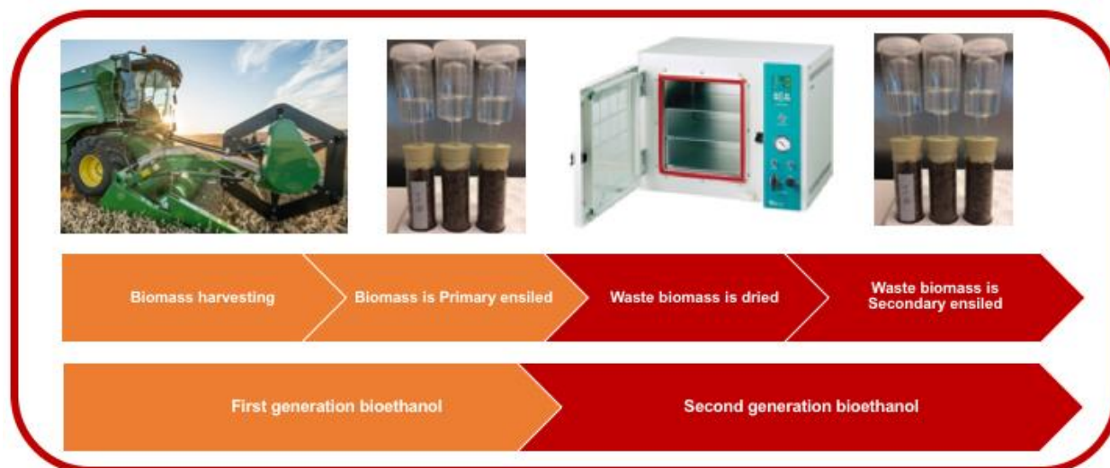
Figure 3. Workflow of Primary and Secondary ensiling laboratory process for production of ethanol
