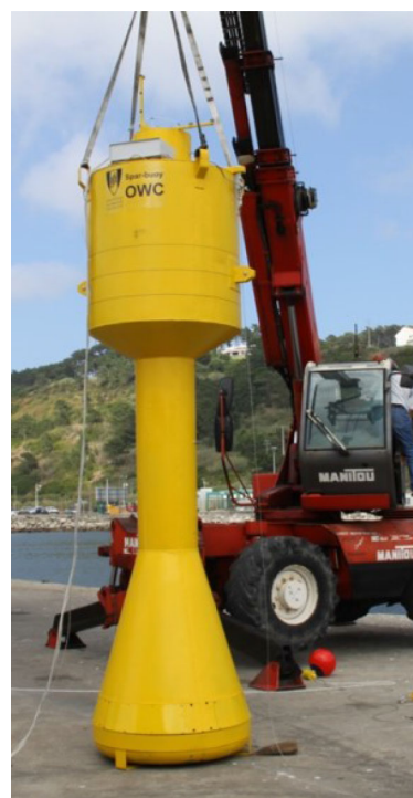
Fig. 3 Spar–Buoy prototype scale 1/16th
