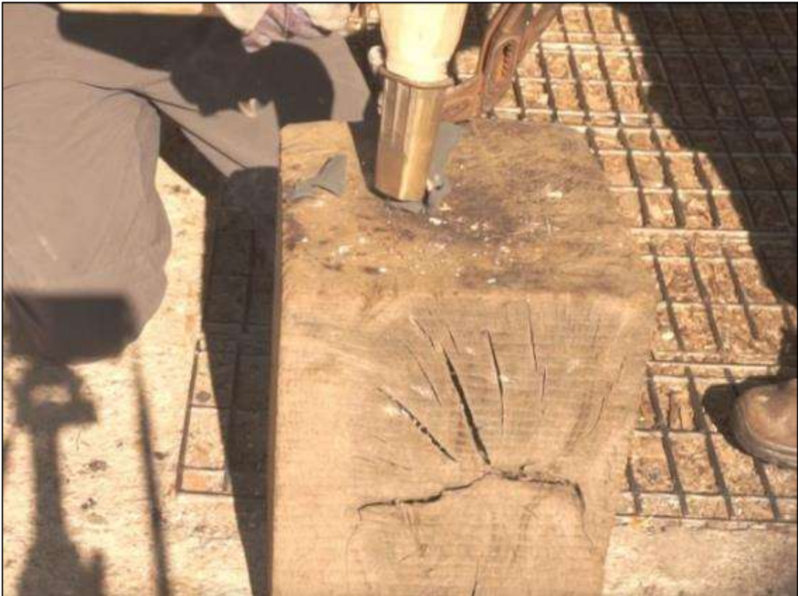
Fig.4.17: Striking the socket end of Axehead 1.3 causing fragmentation (source: Author)
