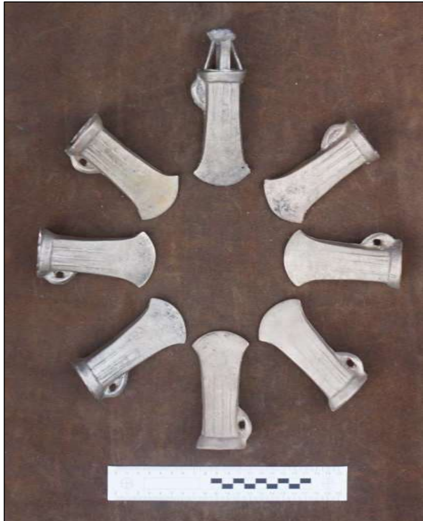
Fig.4.5: The eight replica axeheads produced (1.1-1.8) comprising 3 different compositions (source: Author)
