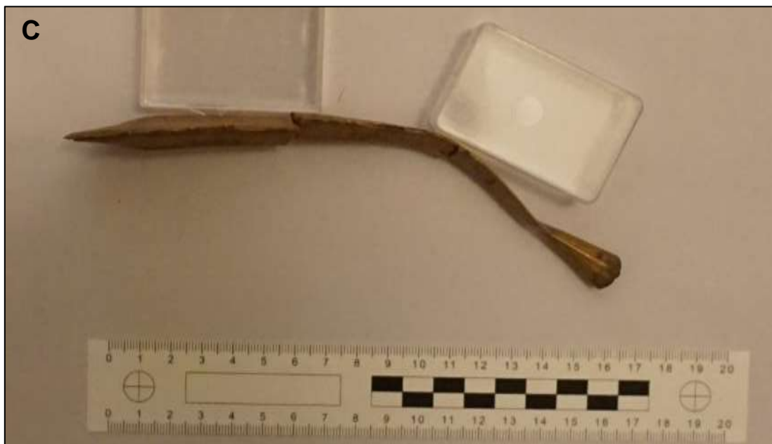
Fig.4.4: An as-cast dagger subjected to fragmentation during Pilot Experiment 1. A) Condition pre-fragmentation; B) The fragmented dagger; C) A side profile showing the transverse bending caused during fragmentation (source: Author)
