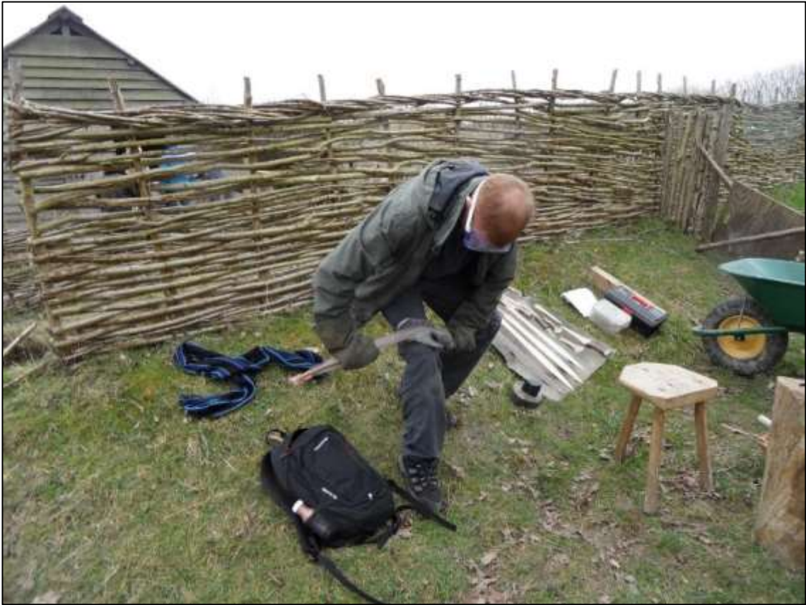
Fig.4.2: The process of bending an as-cast sword by hand in Pilot Experiment 2 (source: Author)
