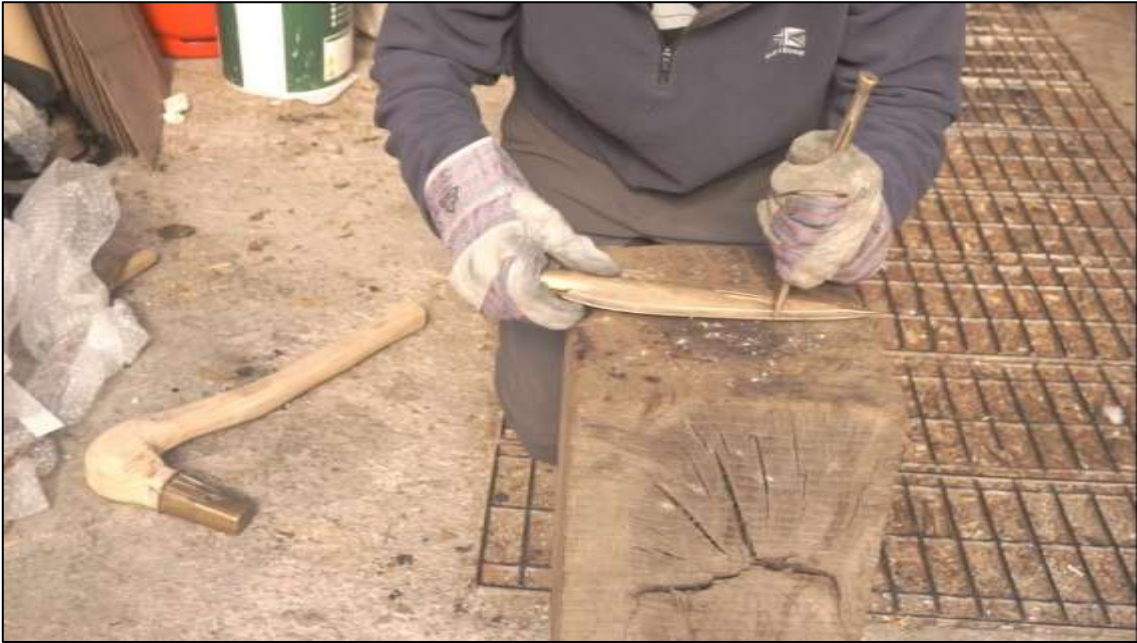
Fig.4.69: Positioning the chisel on Spearhead 3.3 for Experiment 8 (source: Author)
