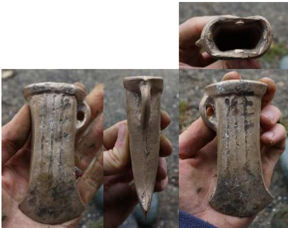
Fig.4.23: Axehead 1.8 after 30 hammer blows (source: Author)
