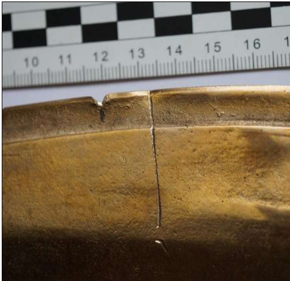
Fig.4.51: A scar left on the flat of Spearhead 3.1 following a sword strike (source: Author)
