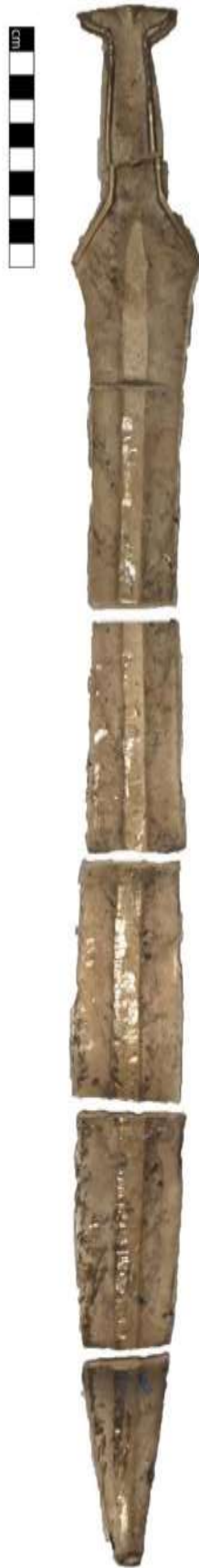
Fig.4.63: Fragmentation of Sword 2.3 after Experiment 6 (source: Author)
