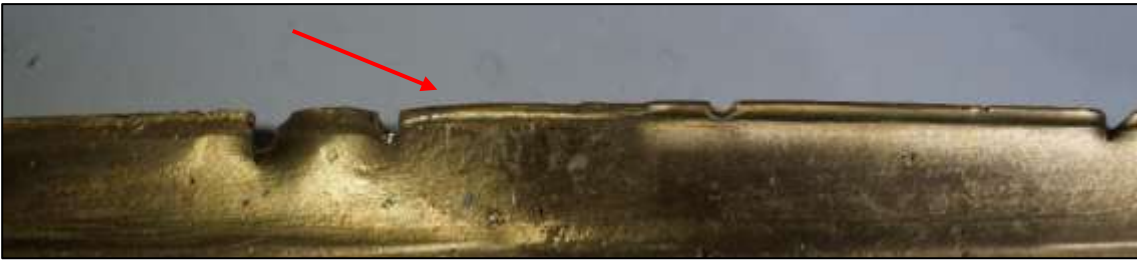
Fig.4.54: The flattened edge of Sword 2.1 after contact with Spearhead 3.1 (source: Author)
