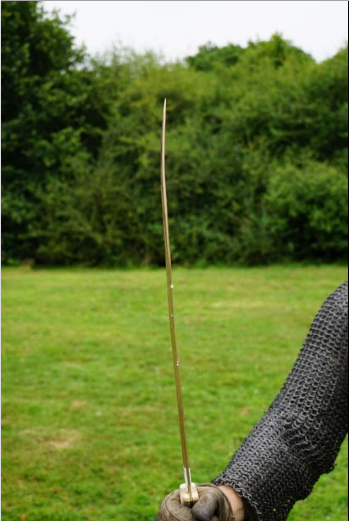
Fig.4.49: Transverse bending on Sword 2.1 after contact with the rim of the shield (source: Author)
