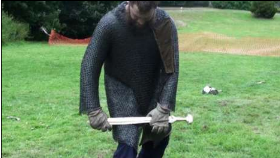
Fig.4.45: Tom Chadwick correcting the bend on Sword 2.1 by applying pressure over his knee (source: Author)
