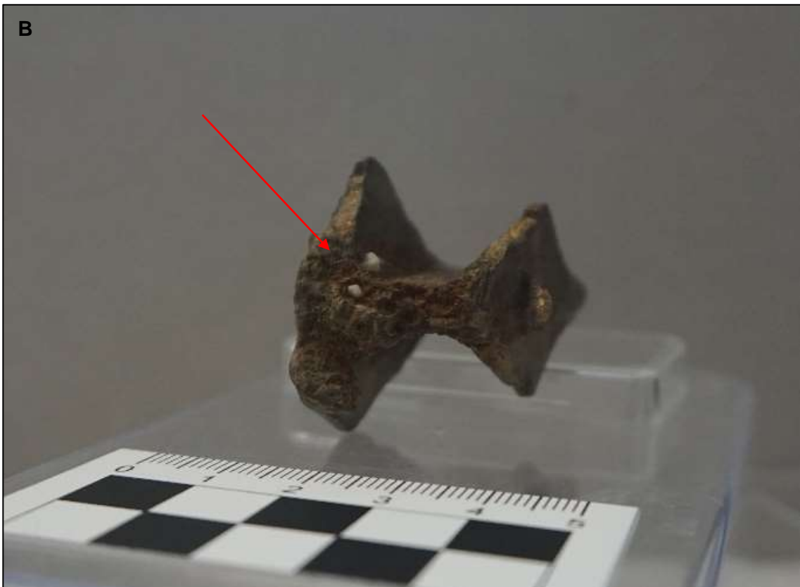
Fig.5.8: Two types of casting flaws causing a break. A shows where an air bubble in the metal has weakened the point of break. B shows where mineral inclusions have become embedded in the metal (source: Author courtesy of the RAMM, Exeter)
