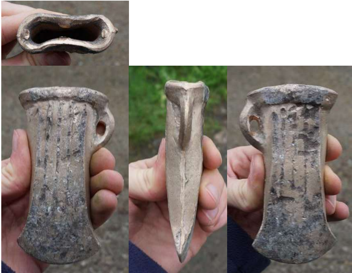
Fig.4.26: Axehead 1.8 after 85 hammer blows (source: Author)
