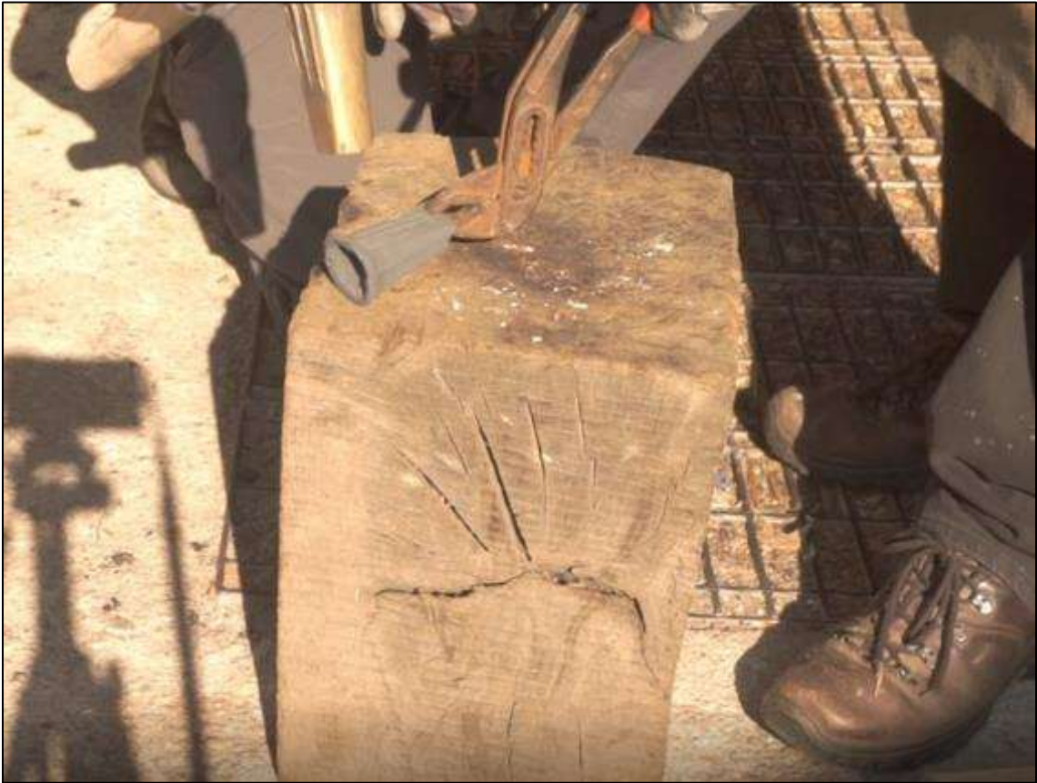
Fig.4.16: Striking the socket end of Axehead 1.6 following separation of the cutting-edge (source: Author)
