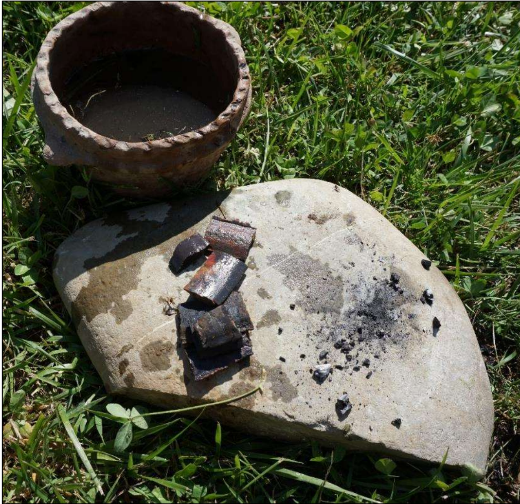
Fig.4.1: Fragments of a deliberately broken sword following casting (source: Author)
