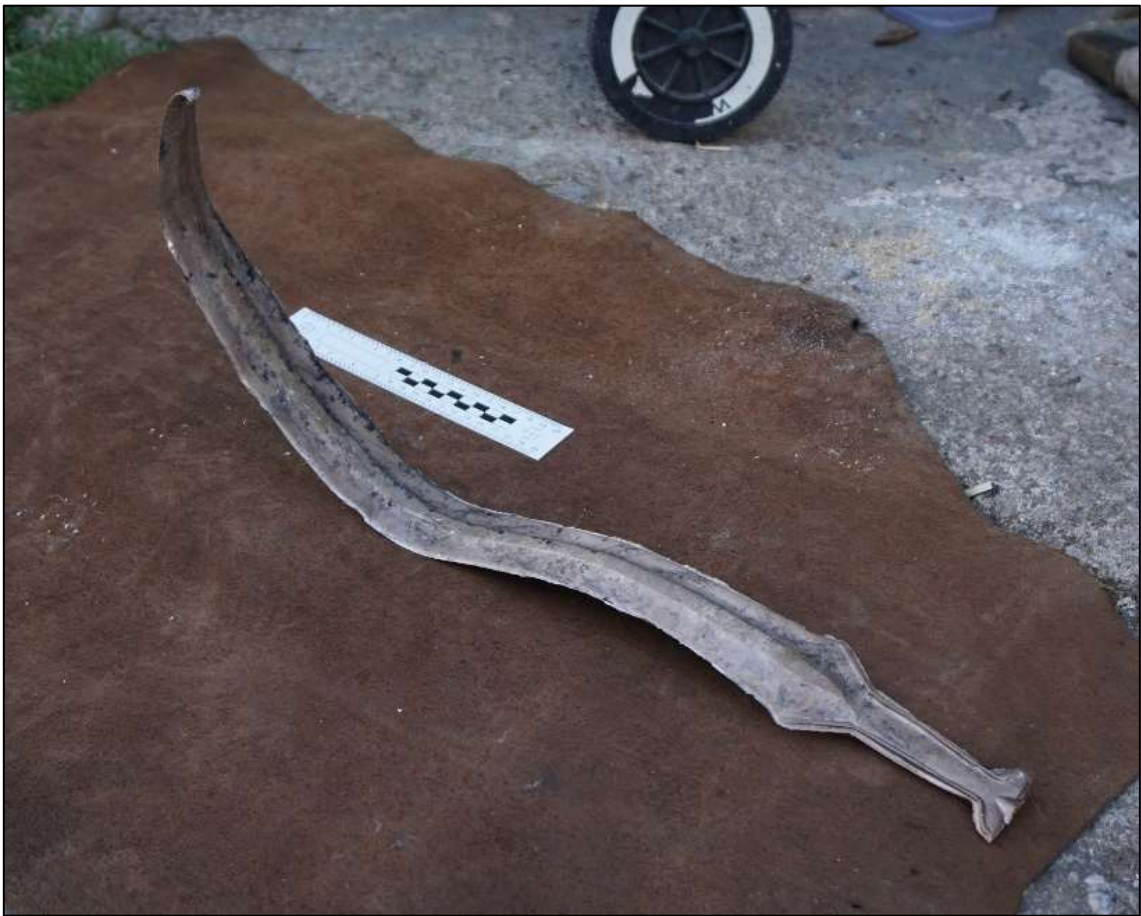
Fig.4.65: Plastic deformation of Sword 2.3 in Experiment 6 (source: Author)
