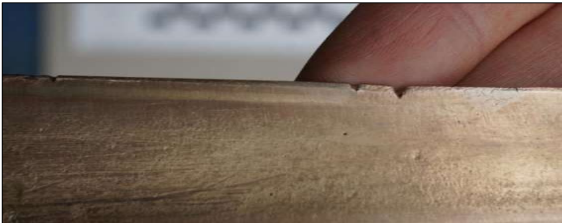
Fig.4.42: Small notches on Sword 2.1 (c.0.5mm deep) (source: Author)
