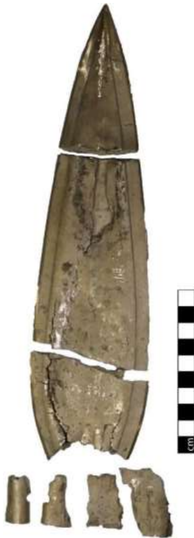
Fig.4.70: Spearhead 3.3 after Experiment 8 (source: Author)
