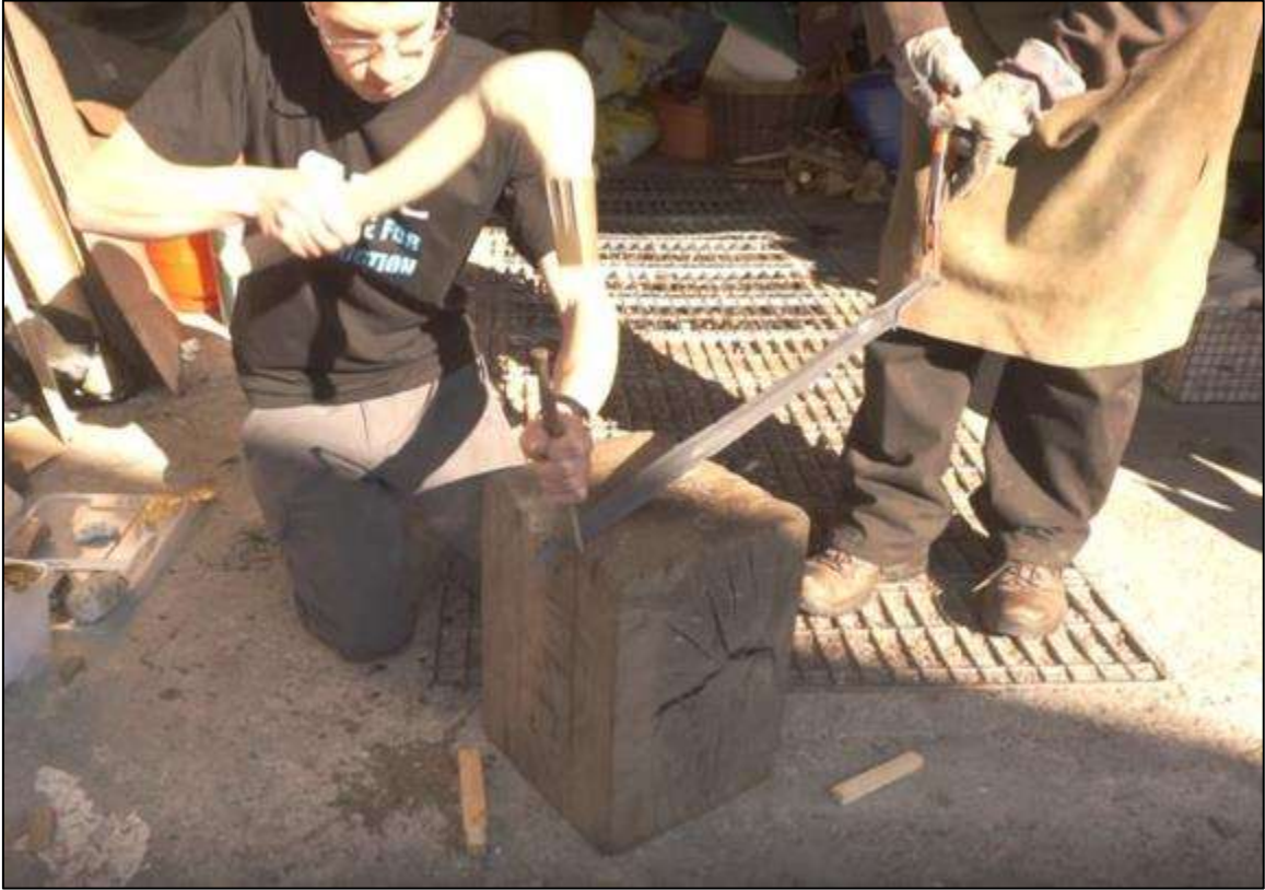
Fig.4.57: Experiment 4 using a hammer and chisel on Sword 2.2 (source: Author)
