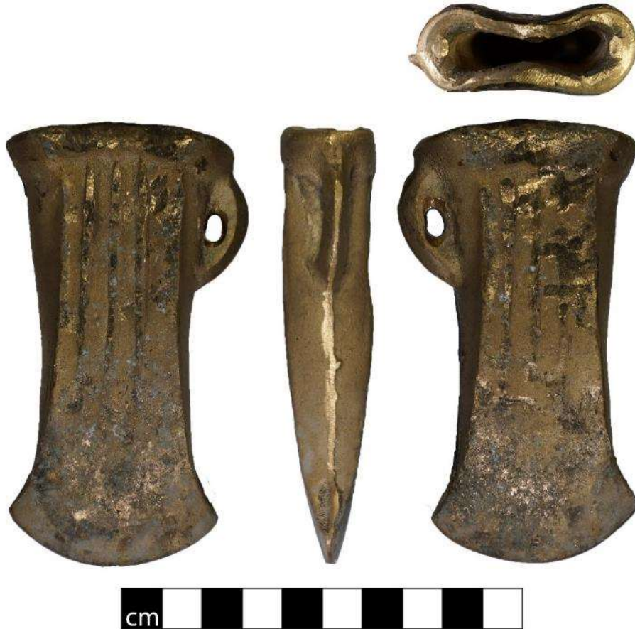
Fig.4.27: Axehead 1.8 after 105 hammer blows (source: Author)
