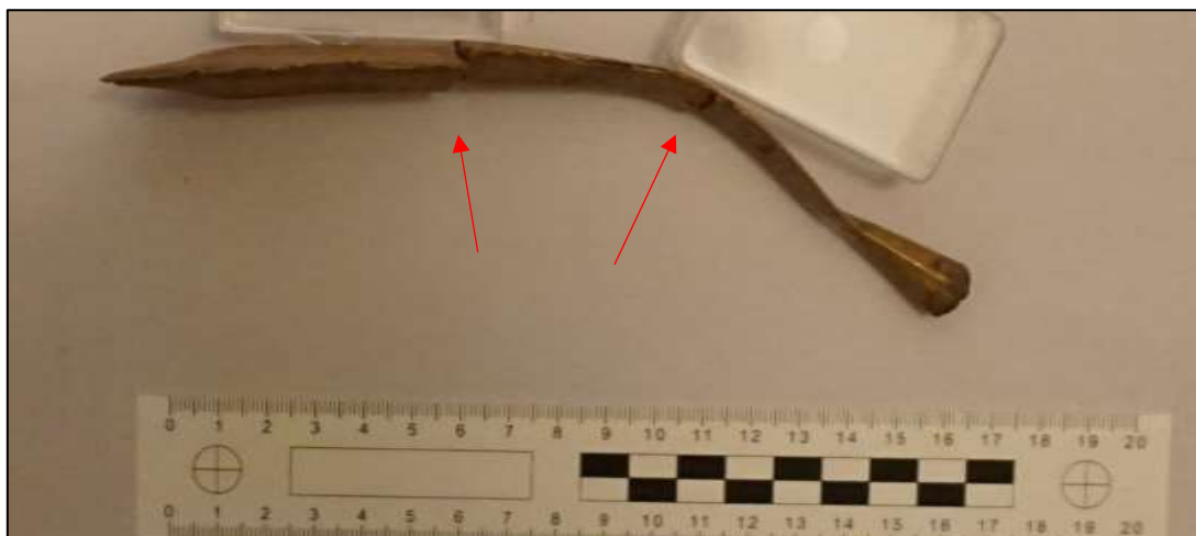
Fig.5.13: A replica dagger broken into three pieces. Arrows indicate the breaking points (source: Author)
