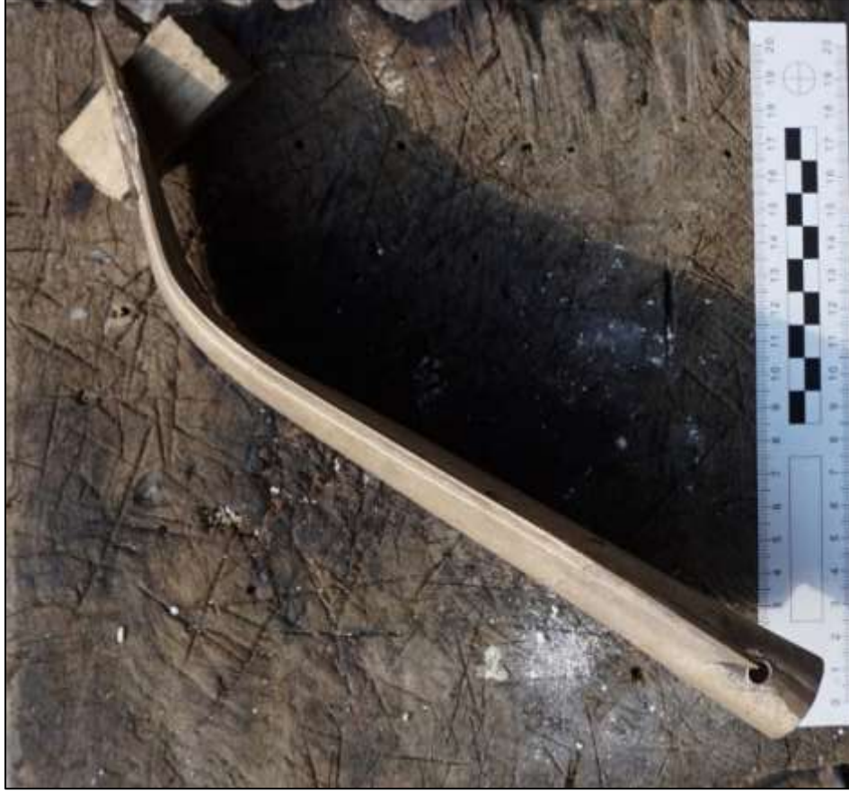
Fig.4.72: Transverse bending of the tip of Spearhead 3.3 after hammering (source: Author)
