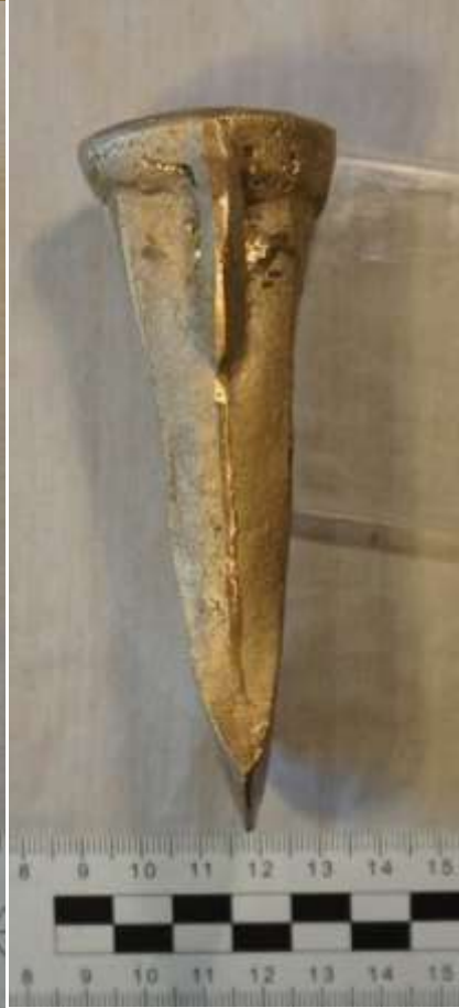
Fig.4.15: Surface damage on Axehead 1.5 following 25 minutes of hammering with a granite hammerstone (source: Author)
