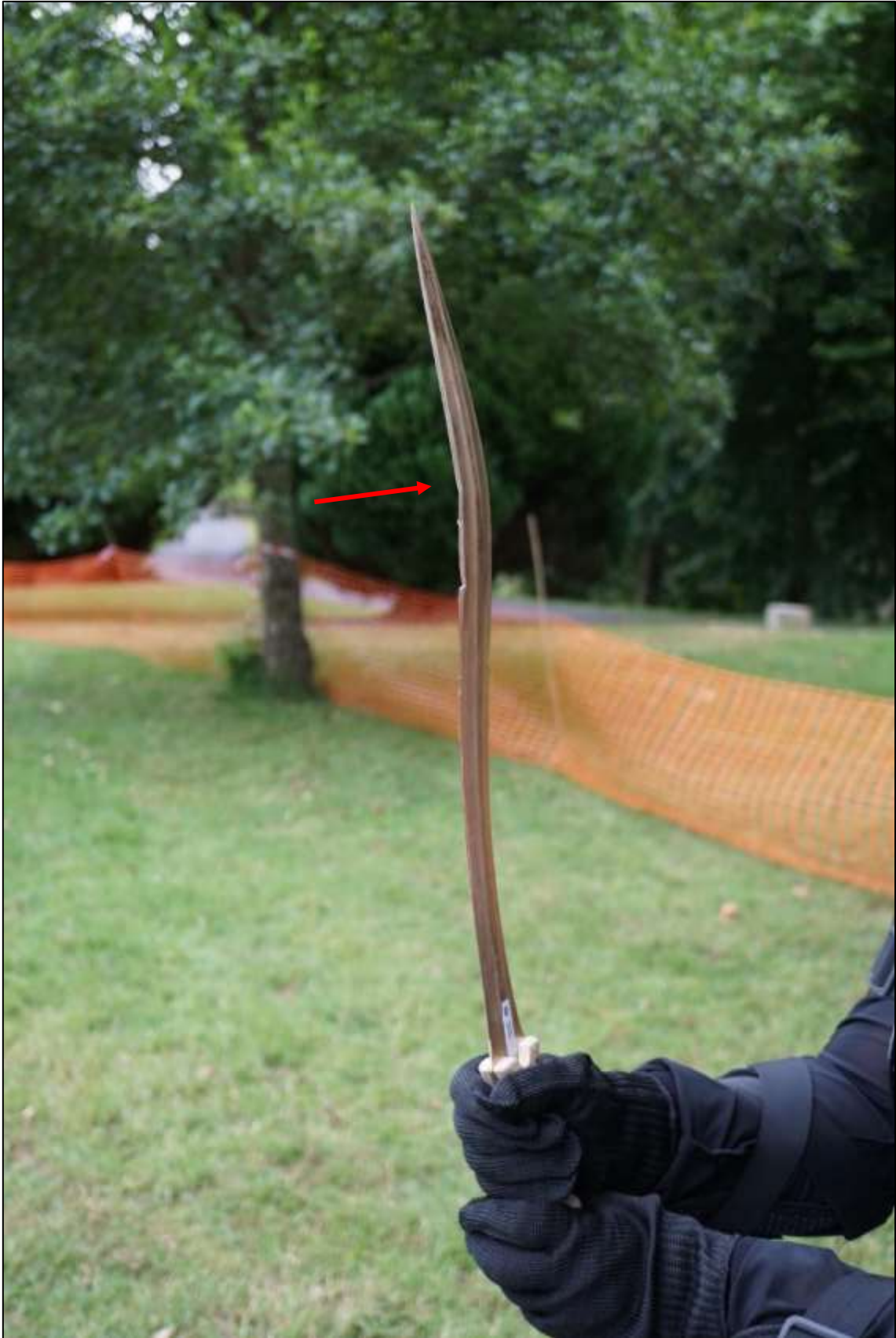
Fig.4.48: Sword 2.2 transversely bent in both directions following a strike to the flat of the blade from Sword 2.1. The arrow indicates the point of contact (source: Author)
