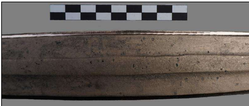
Fig.D.8: One of the edges of Sword 2.1 following hammering (source: Author).
