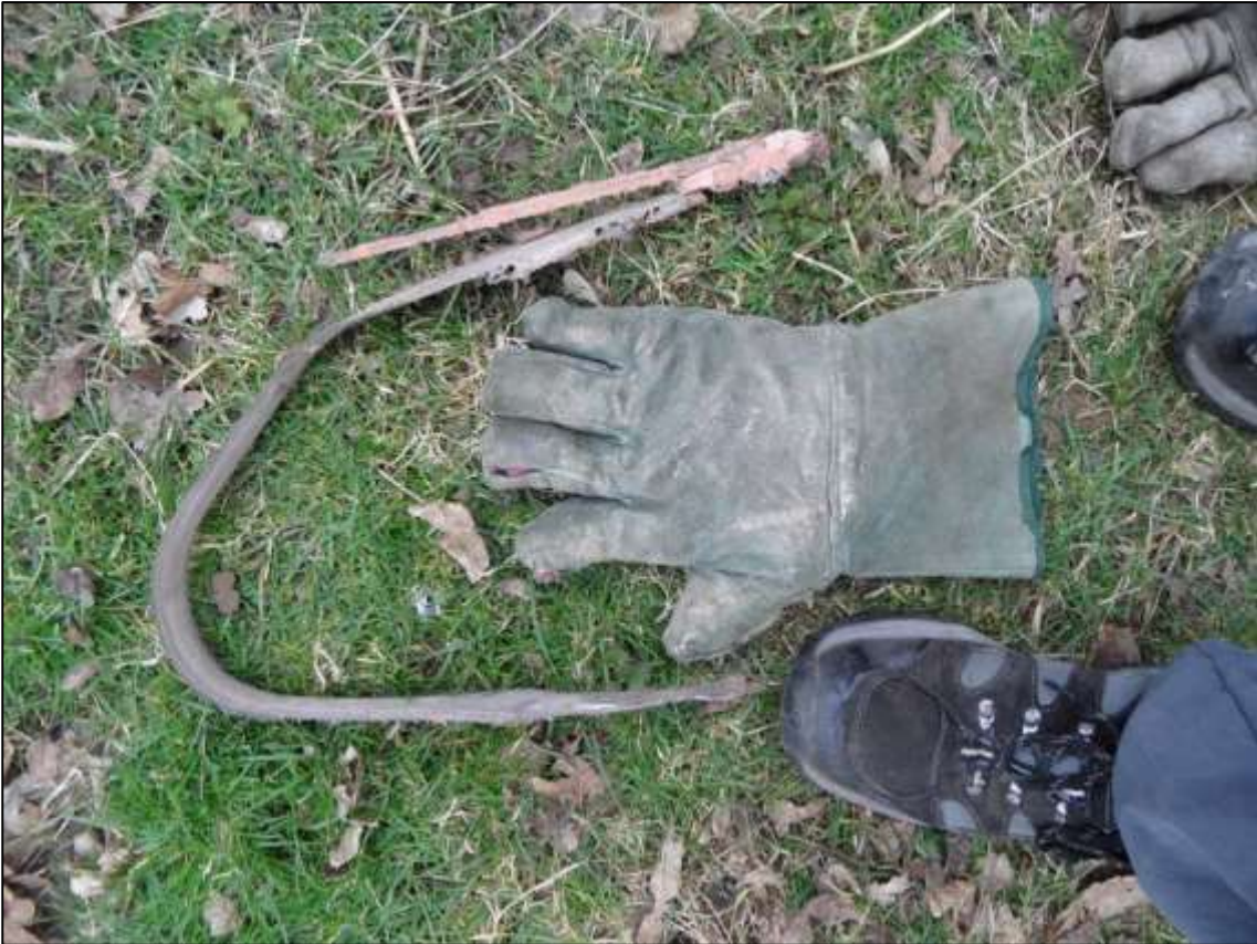
Fig.C.4: The resulting 'u-shaped' bend of the sword in Pilot Experiment 2 (source: Author)
