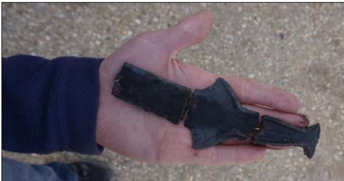
Fig.C.9: Hilt fragments of the tin-bronze sword in Pilot Experiment 5 (source: Author)
