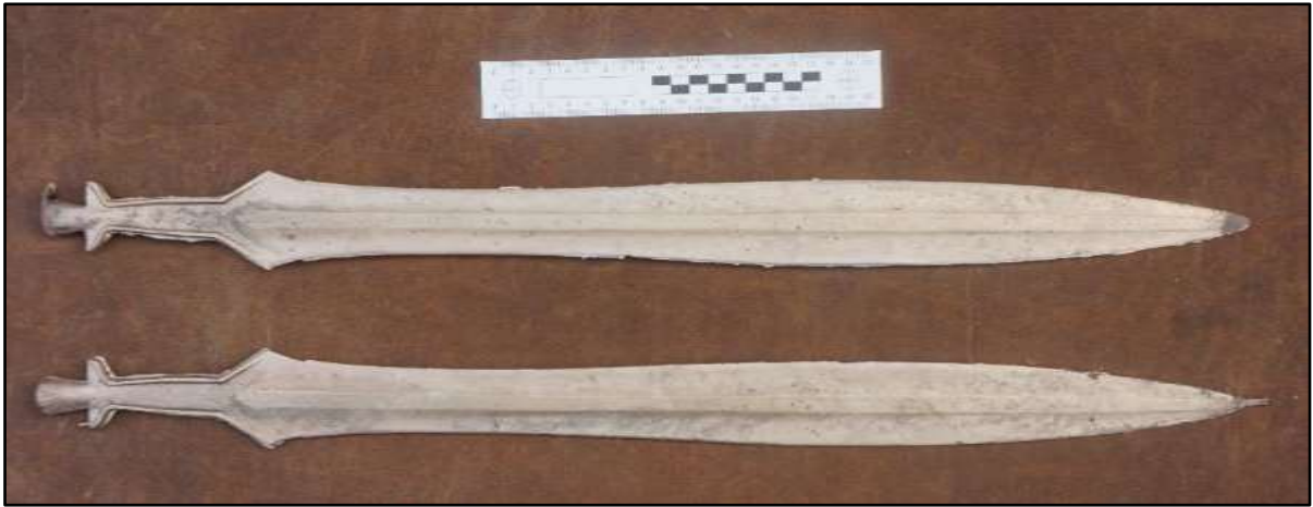
Fig.D.7: The as-cast Swords 2.1 and 2.2 out of the moulds (source: Author).
