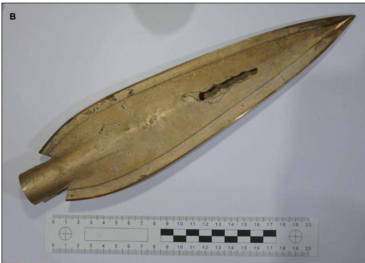
Fig.D.10A: Spear 3.1 at the top, cast without flaws, with Spear 3.2 underneath showing two casting flaws in the blade wall towards the tip (source: author's photo) Fig.D.10B: Spear 3.3 showing a long casting hollow through the blade walls down the midrib (source: author's photo)
