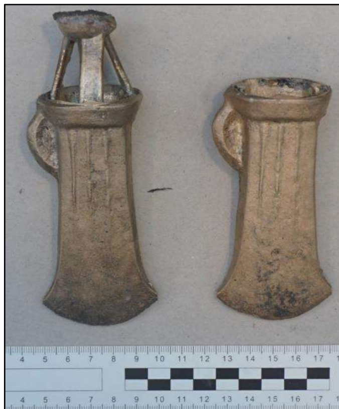
Fig.D.4: Replica Axes 1.2 (15% Sn; 1% Pb) (left) and 1.4 (8% Sn; 2% Pb) (right) demonstrating the difference in colour caused by composition. The higher tin content in Axe 1.2 means it has a slightly more silvery appearance, whereas Axe 1.4 is more yellow. (source: Author)
