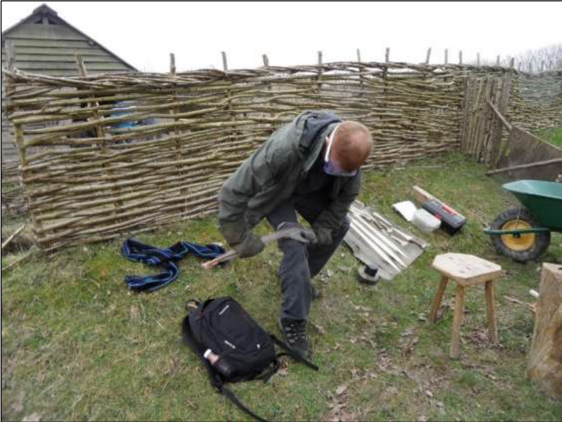
Fig.C.3: Bending the as-cast sword over the author's thigh in Pilot Experiment 2 (source: Author)
