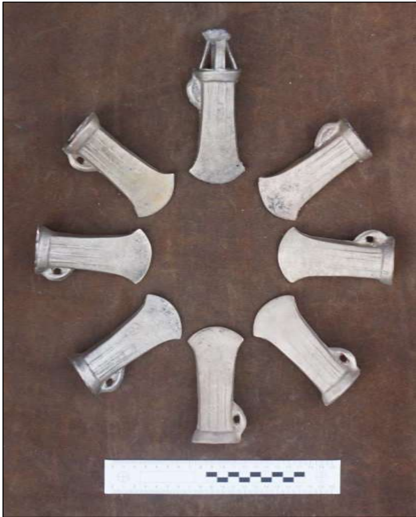
Fig.D.3: The eight replica axes produced (1.1-1.8) comprising 3 different compositions (source: Author)
