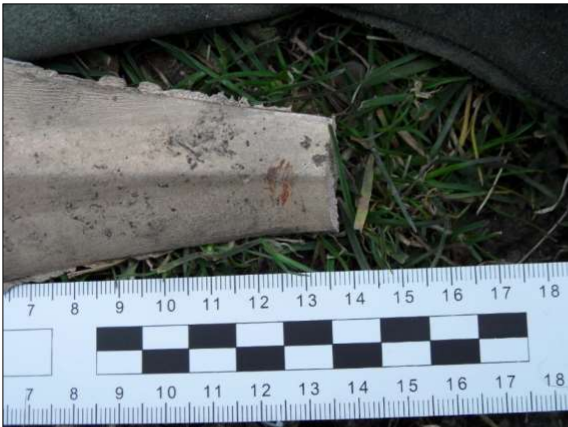
Fig.C.2: The breakage point of the dagger in Pilot Experiment 1 showing no impact mark (source: Author)
