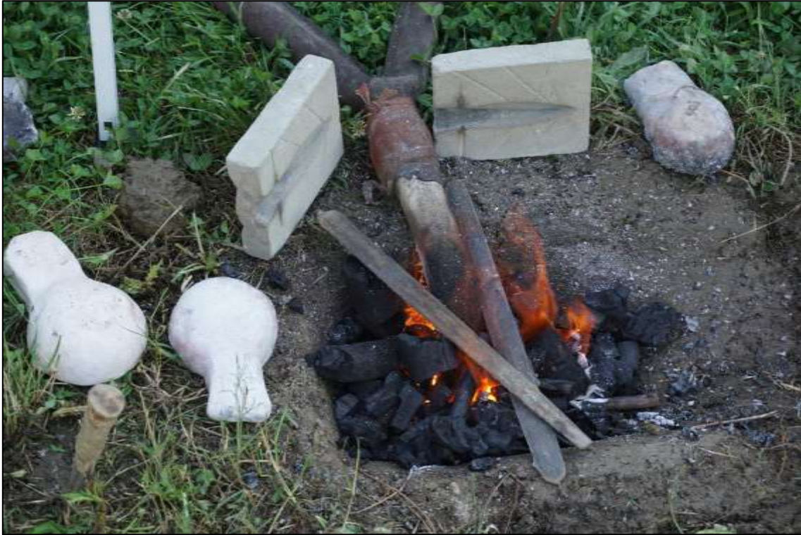
Fig.C.5: Heating swords in the furnace in Pilot Experiment 3 (source: Author)
