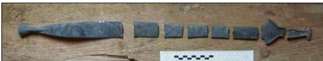
Fig.C.10: The resulting fragments of the tin-bronze sword in Pilot Experiment 5 (source: Author)
