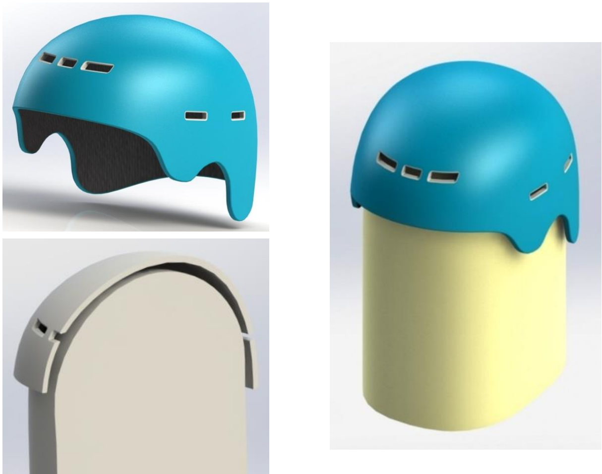
Figure 8: An example of the helmet-head manikin assembly for concept C1
