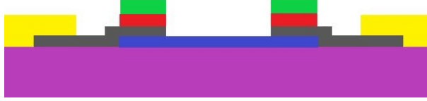
Figure 4.12: Schematic of the proposed contact design for contacting to WSe 2 . With SiO 2 denoted in purple, WSe 2 denoted in blue, graphene in grey, h-BN in red, gold in green and the yellow denotes palladium.
