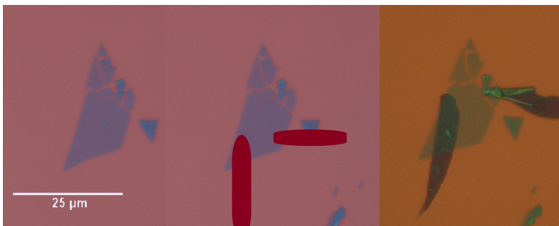
Figure 4.13: Optical micrographs of the MoS 2 flake through the stages of stacking: (a) pristine MoS 2 flake before stacking, (b) desired stacking positions on the flake marked in red, (c) two graphene flakes stacked onto the MoS 2 flake.
