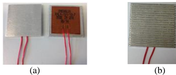
Figure 42: (a) Heating element on top of unfinned Al plate and (b) micro-finned plate.
