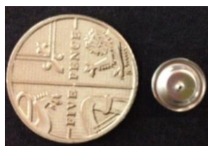
Figure 72: A sealed, pierced lid DSC sample crucible (against a British 5 pence coin for size comparison).
