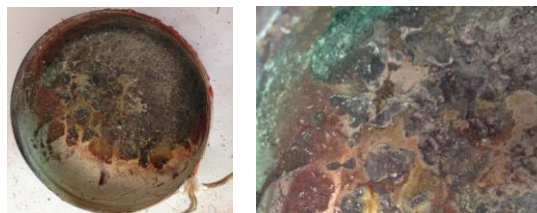
Figure 25: Corrosion of a stainless steel based PCM container.
