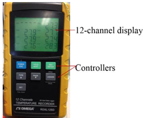
Figure 62: Omega® RDXL12SD 12-Channel temperature recorder front panel.
