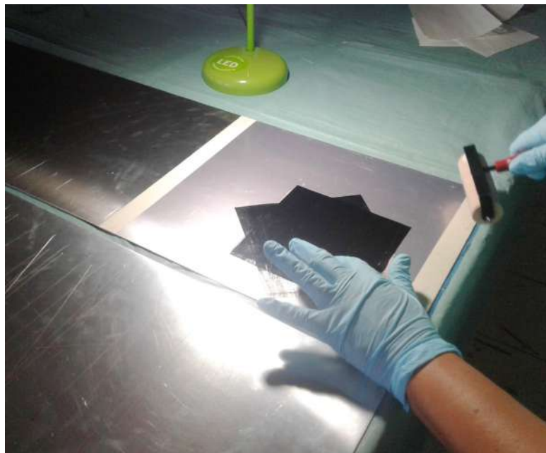
Figure 2: Lay up process for small prototypes. Every CF layer is placed with a 45^\circ angle rotation with respect to the previous one.
