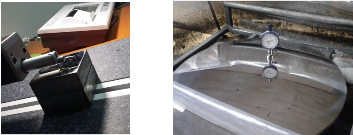
Figure 6: Contact measurement tools. Left panel: Surface roughness tester being applied over a small flat mandrel. Right: spherometer measuring over a 50 cm spherical mandrel. These instruments can measure down to precisions of 10 – 100 nm and 1 \mu\text{m} respectively.
