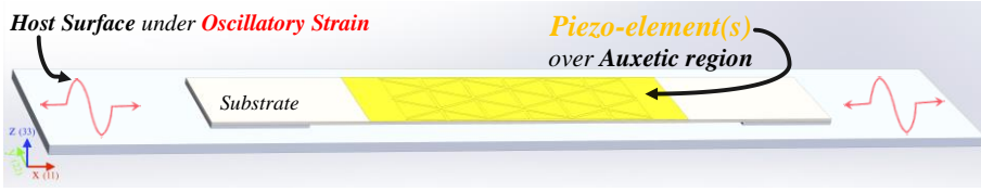
Figure 2: Schematic of the auxetic piezoelectric energy harvester (APEH) bonded over a host structure, the source of vibrations. A second piezo element could be added on the underside of the auxetic region.
