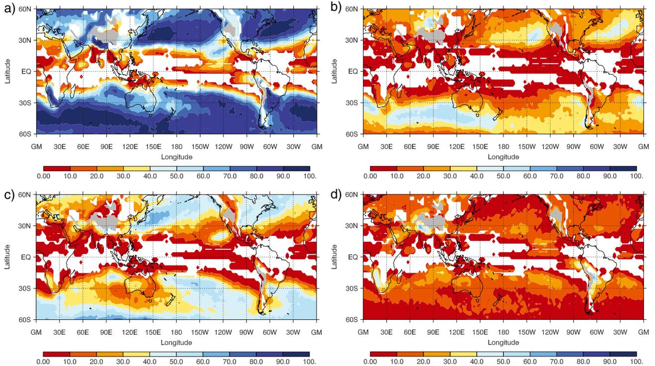
**Figure 3.** The proportion of 6-hourly ERA-Interim extreme precipitation events with a front in the vicinity (1979–2011). (a) All fronts, (b) cold fronts, (c) warm fronts, and (d) quasi-stationary fronts. Regions where the link between fronts and precipitation is not statistically highly significant are blanked out in white and high orography is blanked out in grey.
