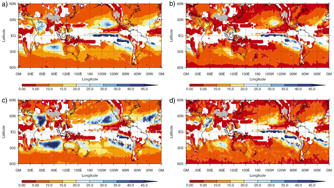
**Figure 5.** The proportion of fronts that lead to 6-hourly ERA-Interim extreme precipitation events (1979–2011). All fronts (a), cold fronts (b), warm fronts (c), and quasi-stationary fronts (d). Regions where the link between fronts and precipitation is not statistically highly significant are blanked out in white and high orography is blanked out in grey.
