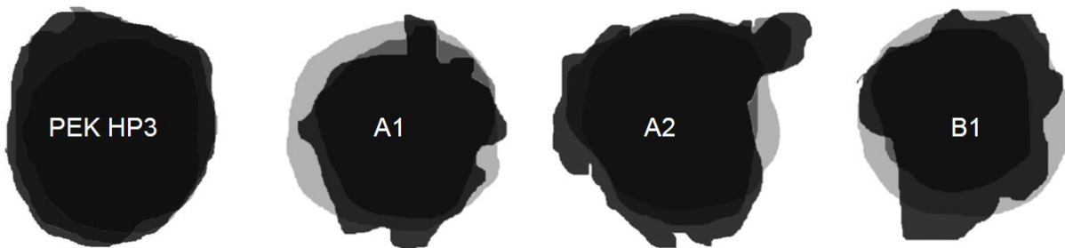
Figure 11: Change in particle size with temperature. The darkest image corresponds to the particle at room temperature, followed by the particle at (T)^\circ\text{C} and the lightest colour corresponds to the particle at T_{\text{max}}
