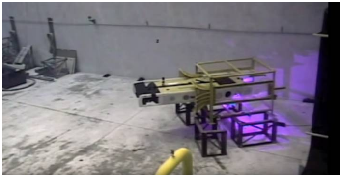
Figure 5. Saab Sabretooth Class VIB vehicle being tested with a subsea garage at NASA Neutral Buoyancy Laboratory (Saab 2015).
