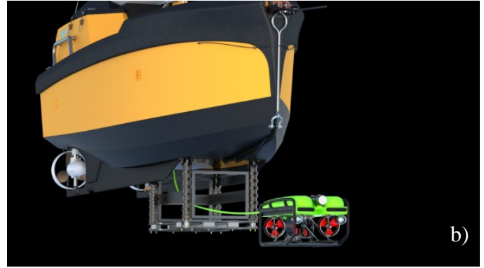
Figure 12. ASV C-worker 7 vessel shown deploying an ROV via a frame through the moonpool. a) side view b) elevation view
