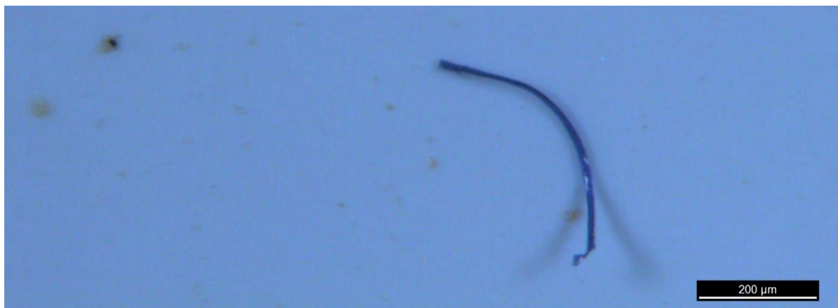
Figure 2.5: Example of a microplastic fibre found in a seawater sample.
