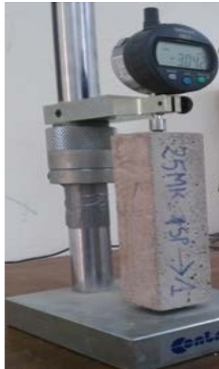
Figure 6. Total shrinkage test.
