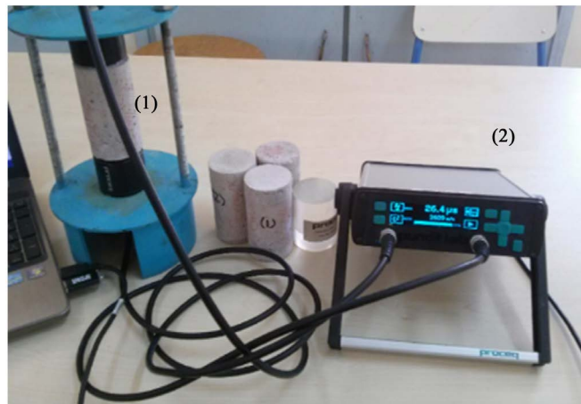
Figure 8. Ultrasonic pulse velocity testing experimental setup-Pundit: (1) tested specimen between transducers on the experimental setup; (2) Pundit apparatus digital pulse recorder.
