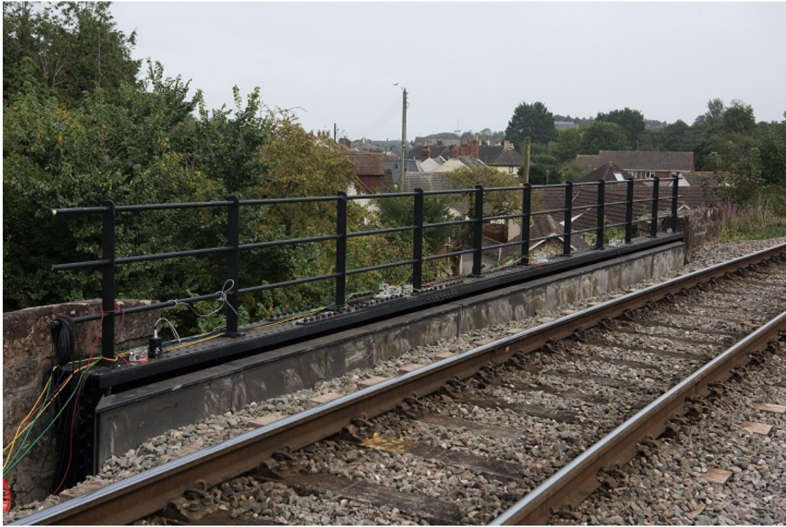
Figure 4: Layout of the accelerometers on the deck
