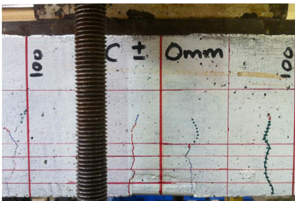
Figure 13: Crack heights at the mid-span of RC Beam 1 (3.72 kN load).
