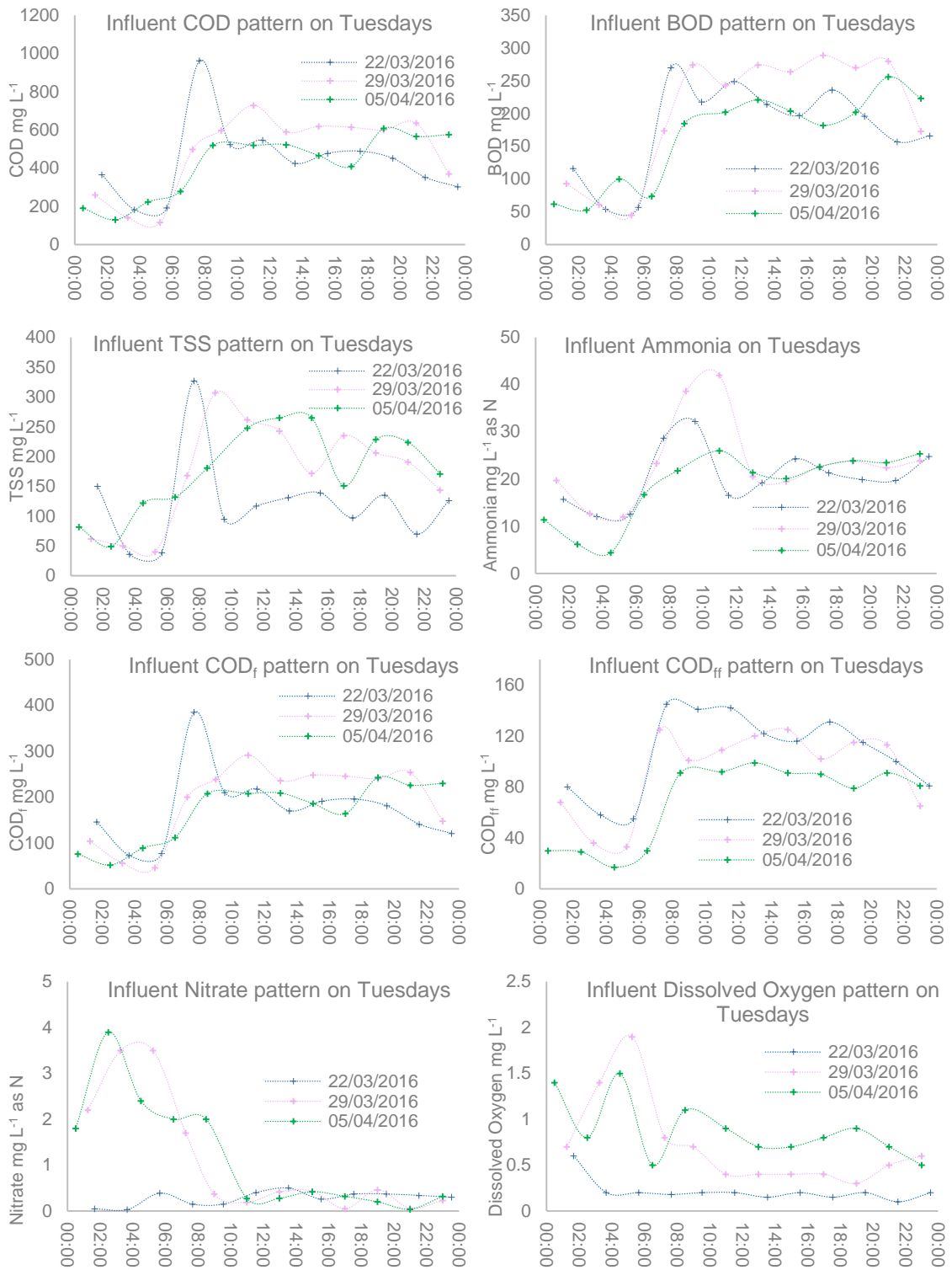
Figure A-2: Influent wastewater pollutants pattern from samples in the campaign period on Tuesdays
